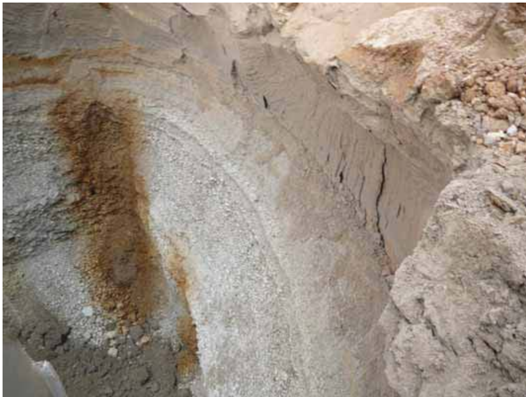
Test Pit C Lower strata – Coarse pumice (6.0 – 9.5 m+) below thick layer of Pumicite
