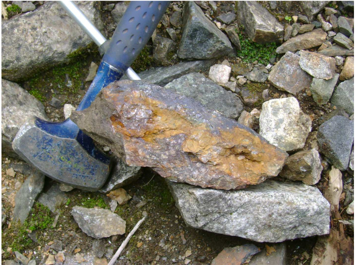
Plate 2 -Vein breccia (Mo-68&69) up to 418 g/t Ag, 0.1% Cu, 0.54% Pb, 0.14% Zn
