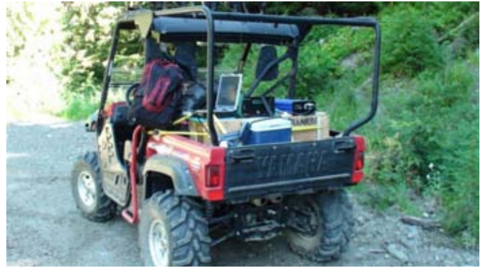
Figure 4, GR460 Mobile Spectrometer System Installation Spectrometer Data Display Spectrometer System Mounted in Rhino
