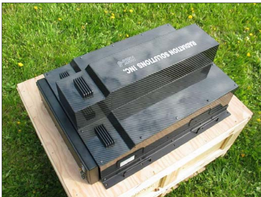
Figure 6 - Radiation Solutions RSX-5 Gamma Ray Spectrometer.
