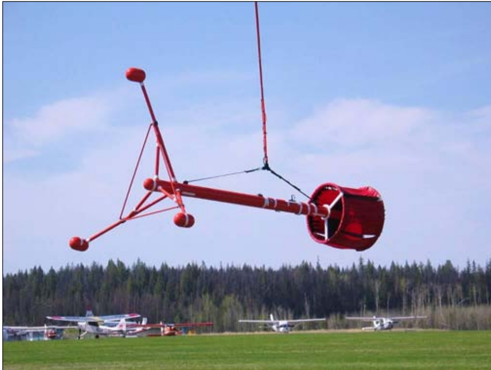
Figure 5 - The CMG tri-axial magnetic gradiometer.
