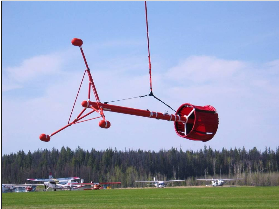
Figure 5 - The CMG tri-axial magnetic gradiometer.
