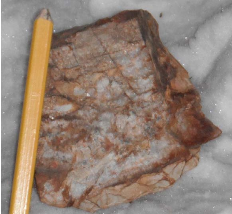
Photo 4-2: Quartz vein breccia (with albite, goethite and galena), sample SKKG-113 assaying 7.8 g/t Au (note snow in background).
