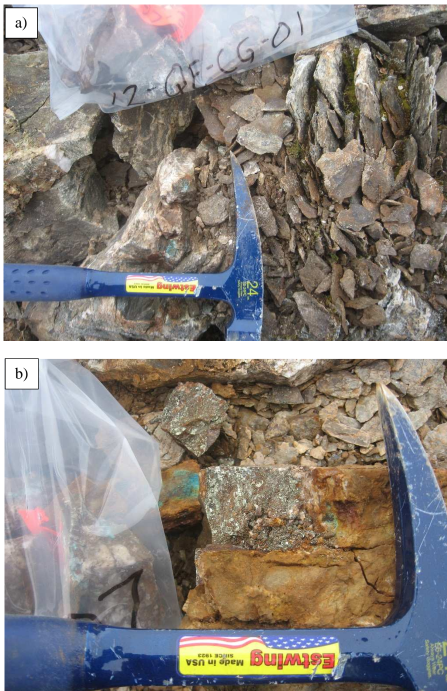
Figure 7. a) Schistose rocks are common at Site A; Sample 12-QE-CG-01 exhibits malachite staining and contained 207 ppb Au; b) Sample 12-QE-CG-07, which contained 30.7 g/t Au, 159 g/t Ag, 4.47% Cu.
