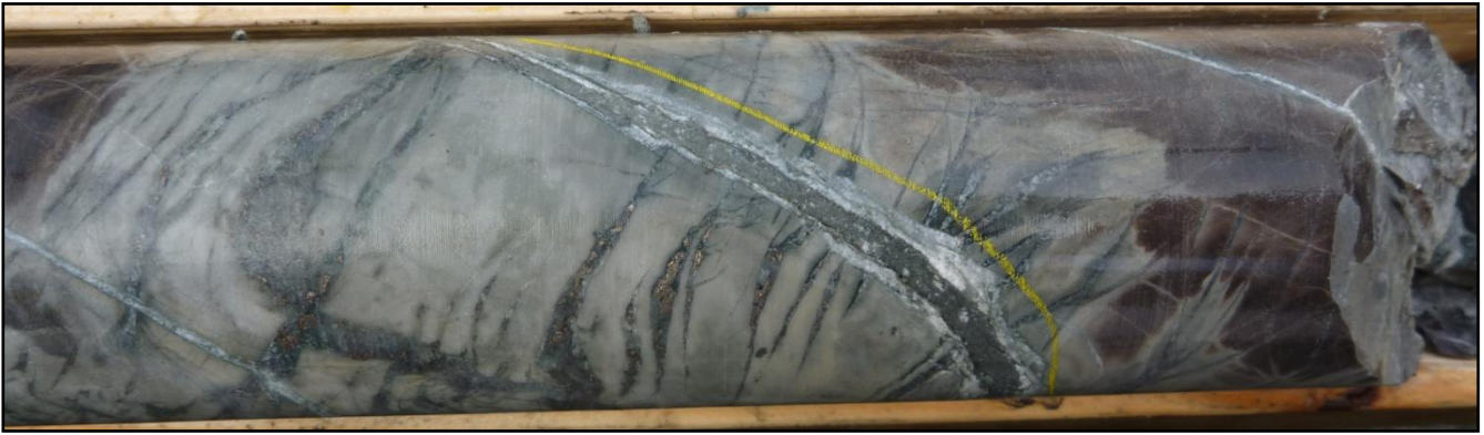
Plate 1. Core photograph of drill hole JSP12-003 at 541.5 m depth. Piece of core in view is approximately 15 cm in length. A minor pyrite/pyrrhotite/quartz breccia structure occupies a calcite veinlet marked by the yellow line. Pyrrhotite-chlorite lenses are cut by this structure and typical albite/chlorite retro-grade alteration can be seen to propagate from the fractures and lenses into the biotite hornfels.
