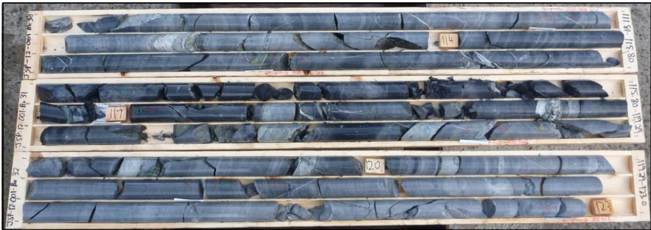
Plate 1. Core photograph of drill hole JSP12-001 from 111.81 m to 123.0 m. Zone of high Mo (1030 ppm) occurs from 115 m to 117 m in the central area of the photograph, correlating with a moderately broken section of fine grained black hornfelsed calcareous sediments surrounded by pale calc-silicate hornfels. Minor calcite veining and fractures throughout.
