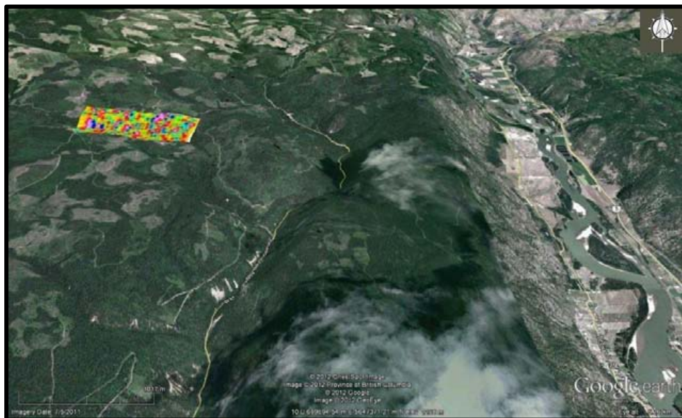
Figure 6. Contoured VLF-EM Data Fraser Filtered on Google (Note the deeply incised river valley structure and the parallel and the northwesterly structures to the west)
