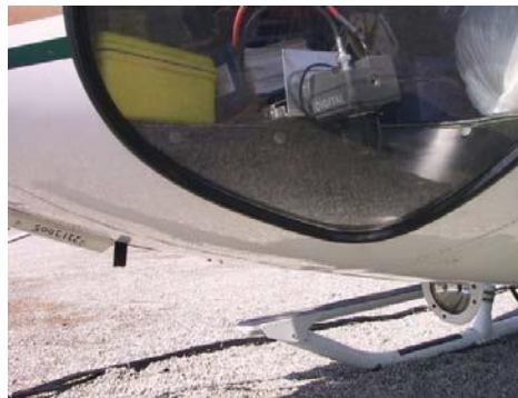
Figure 4.: Digital video camera typical mounting location
