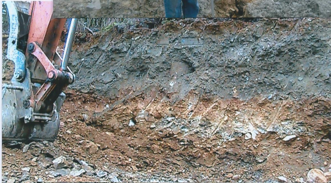
glacial #2 clay overburden Red ancient tertiary Channel #10/m 3 Argillite Bedrock
