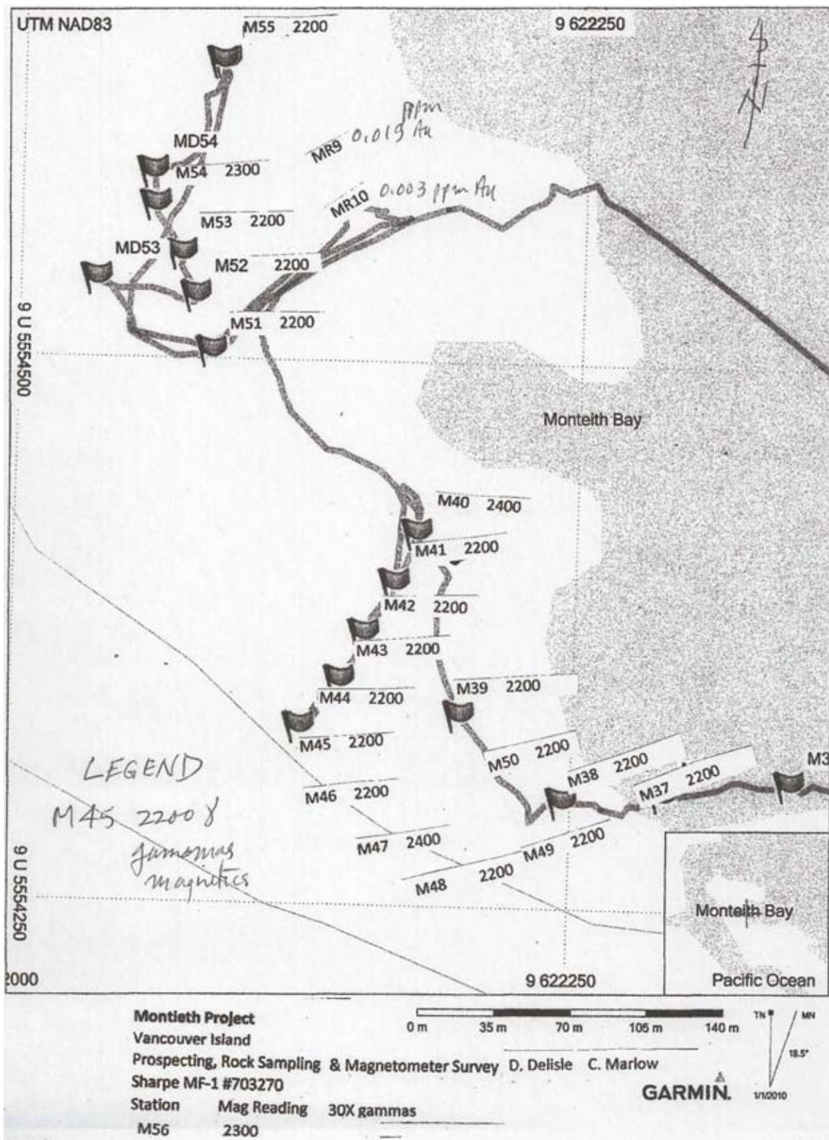
Figure 9 Magnetometer Results and Soil Results, West Side
