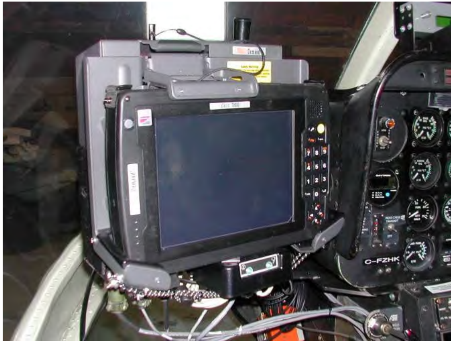
Figure 12: AGIS installed in the Bell 206.
