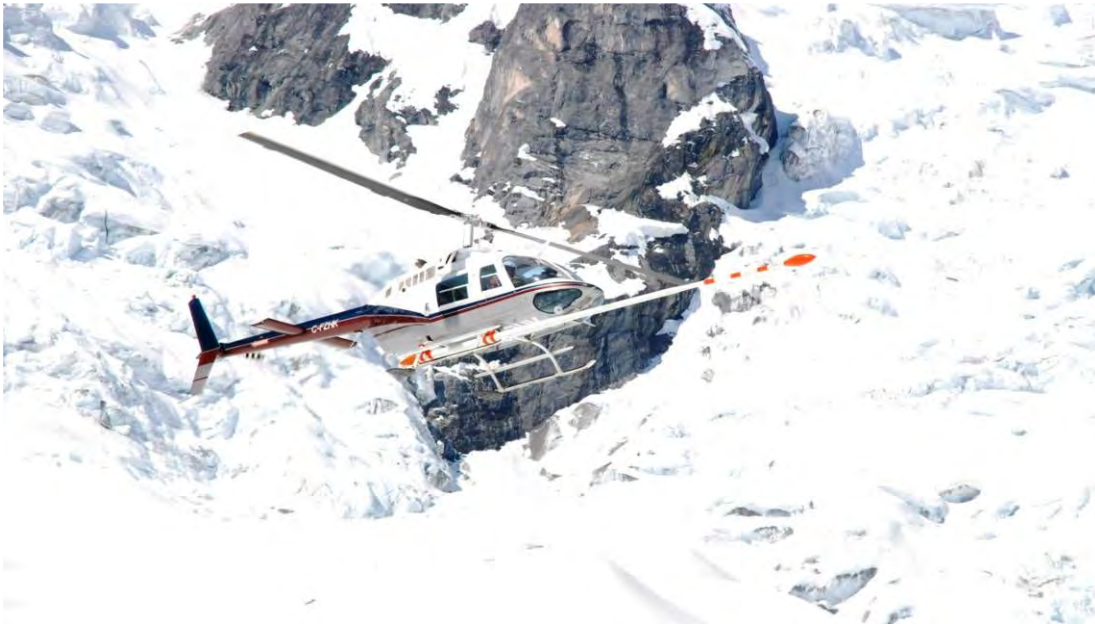
Figure 11: Bell 206 Jet Ranger equipped with mag stinger for magnetic data acquisition.
