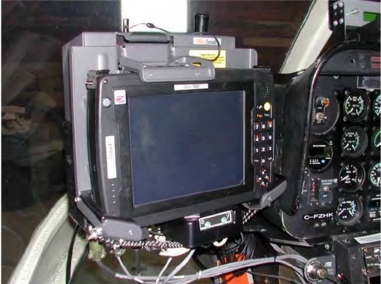
Photo 1: AGIS installed in the Bell 206
