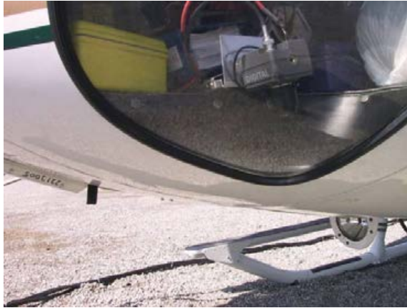
Figure 6: Digital video camera typical mounting location.
