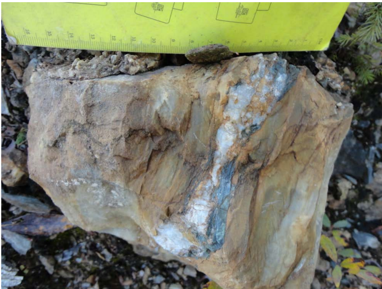
Photo 2.0: Calcitic limestone/marble (brown) with quartz vein and an interbed of slate(?) (dark green).
