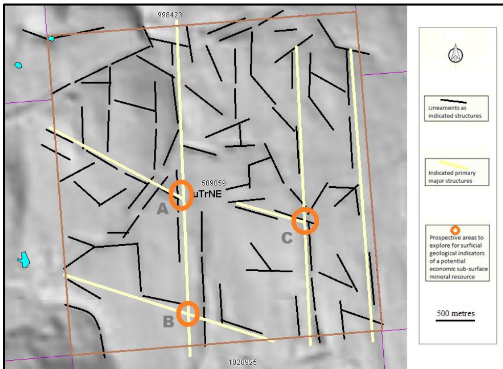
Figure 7. Lineaments as Indicated Structures on Tenure 589859
