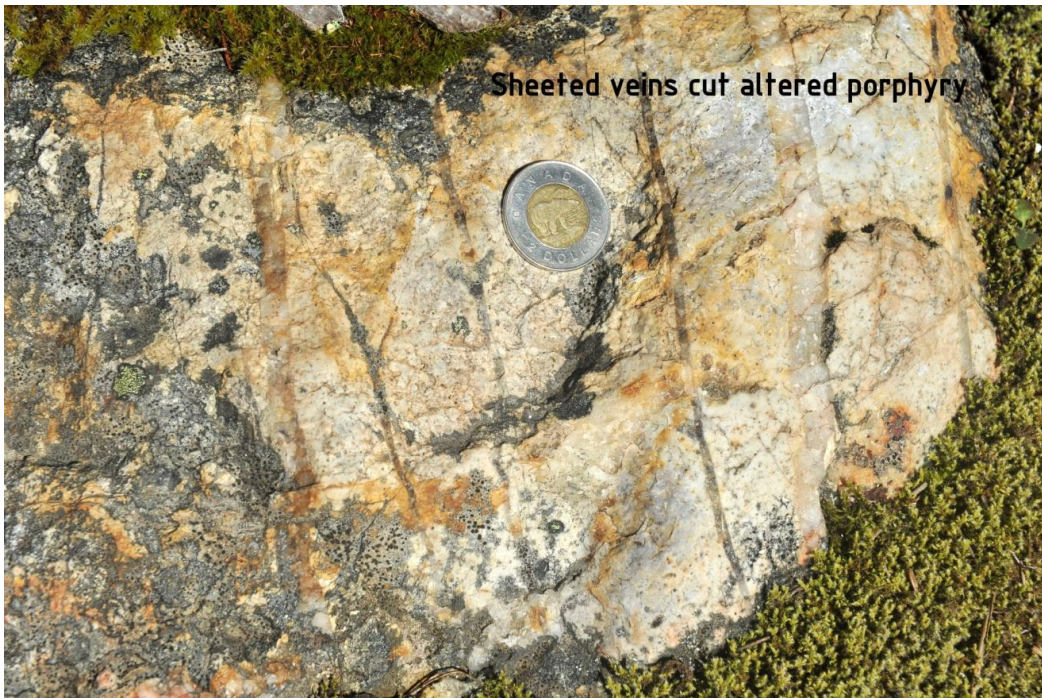
Figure 8.14: Cm-scale, parallel, late quartz veins filled by translucent to pale grey quartz. These veins are thought to host gold.
