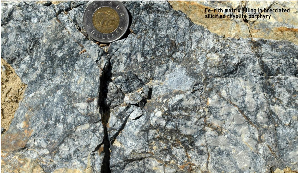
Figure 8.8: Silicified rhyolite porphyry brecciated and infilled by dark grey iron-rich(?) siliceous matrix.
