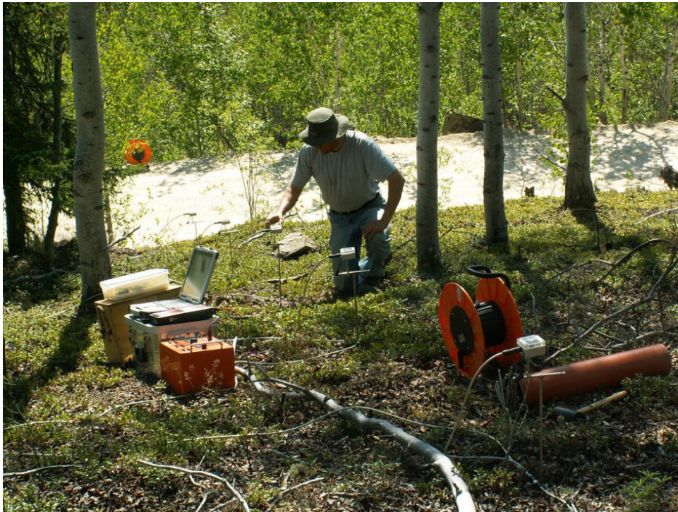
Figure: 2D Resistivity measurement, Stefan Ostermaier, Arctic Geophysics Inc., Yukon 2009
