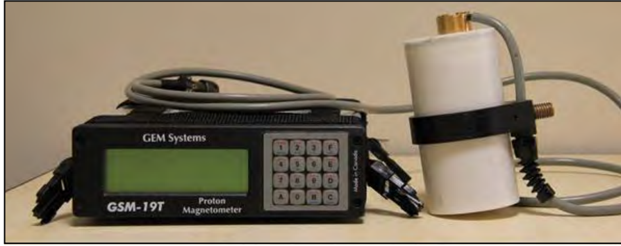
Figure 13: GEM GSM-19T proton precession magnetometer.
