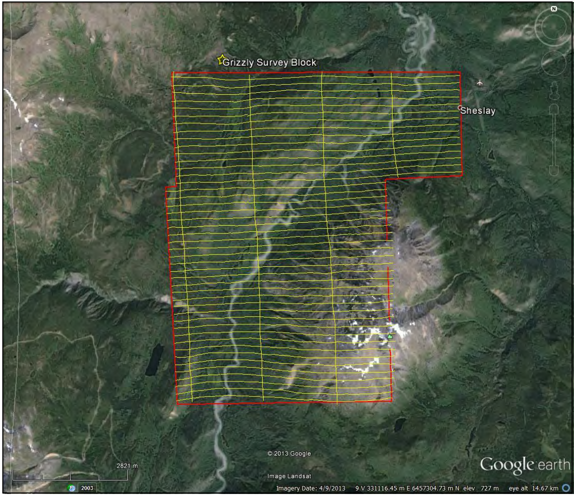
Figure 4: Plane View – Grizzly survey block with actual survey and tie lines outlined in yellow, and the survey block boundary in red.
