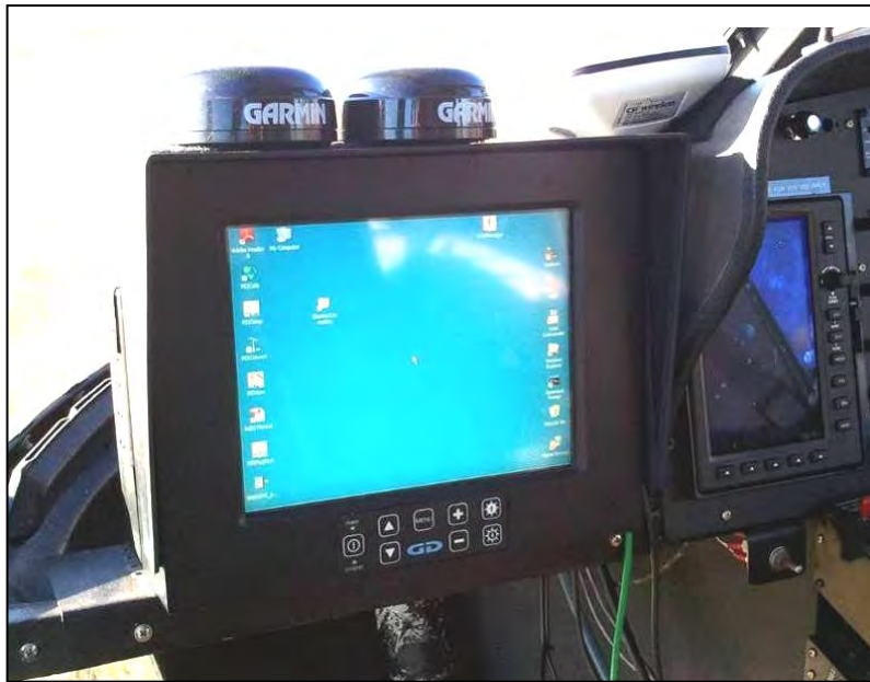
Figure 10: AGIS operator display installed in the Eurocopter AS350B2.
