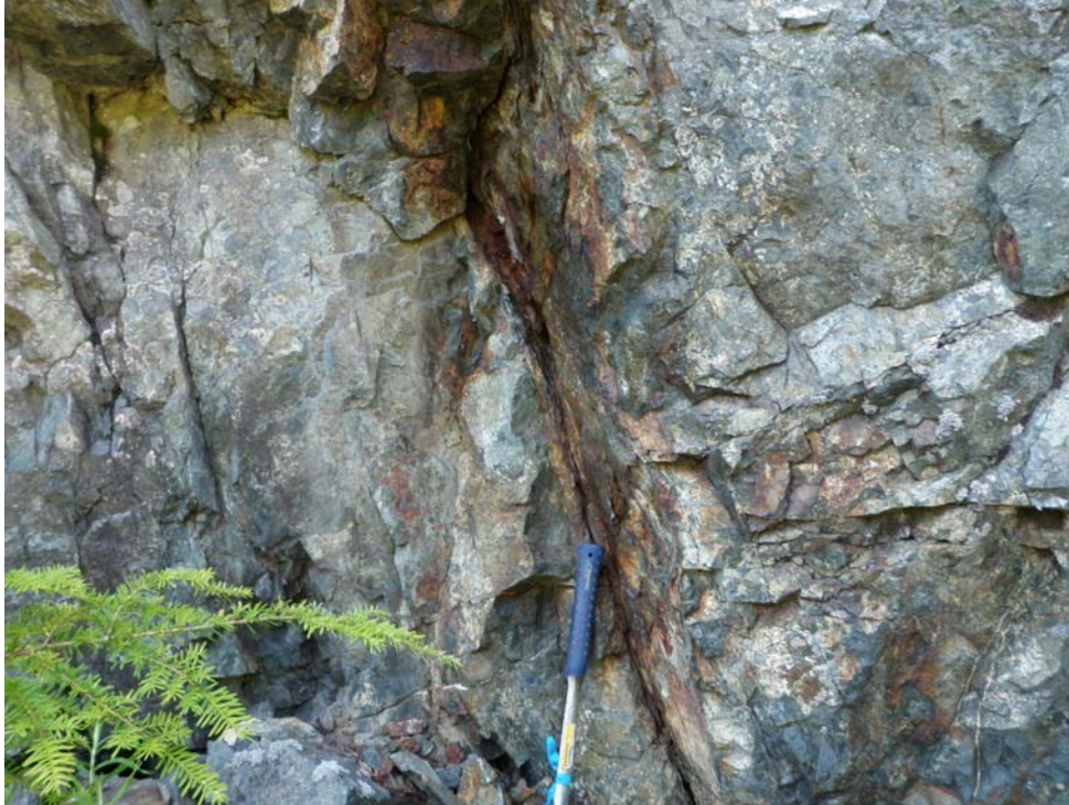
Photo 1: zone of strong chlorite alteration carrying veinlets and fracture fillings of pyrite-chalcopyrite-bornite; WP190; sample 1615102
