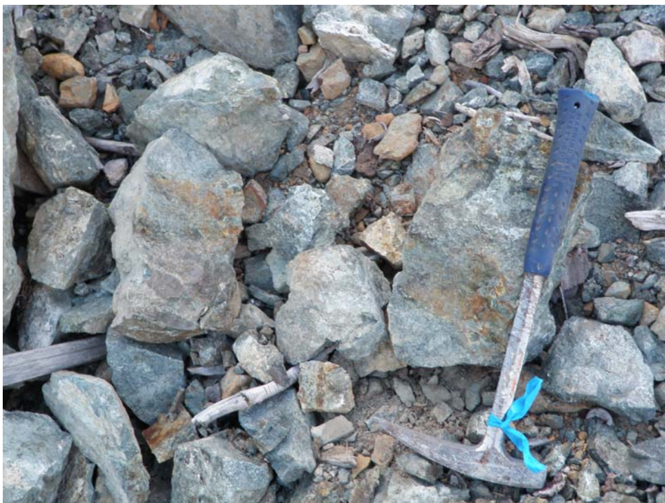
Photo 2: silicified basalt rubble with epidote-calcite-pyrite-chalcopyrite veinlets; WP191; sample 161103
