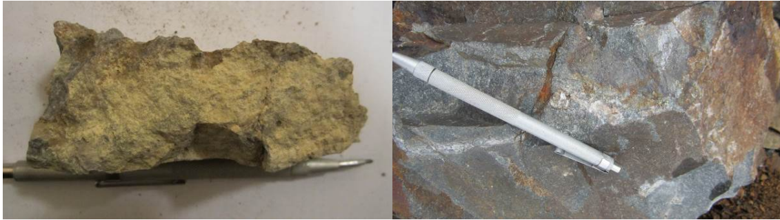
Photo 20, L. Sample 300A – Suspected phlogopite with strong overprinting of jarosite. Photo 21, R. Quartz-pyrite±chalcopyrite vein observed in monzodiorite (Sample 302).
