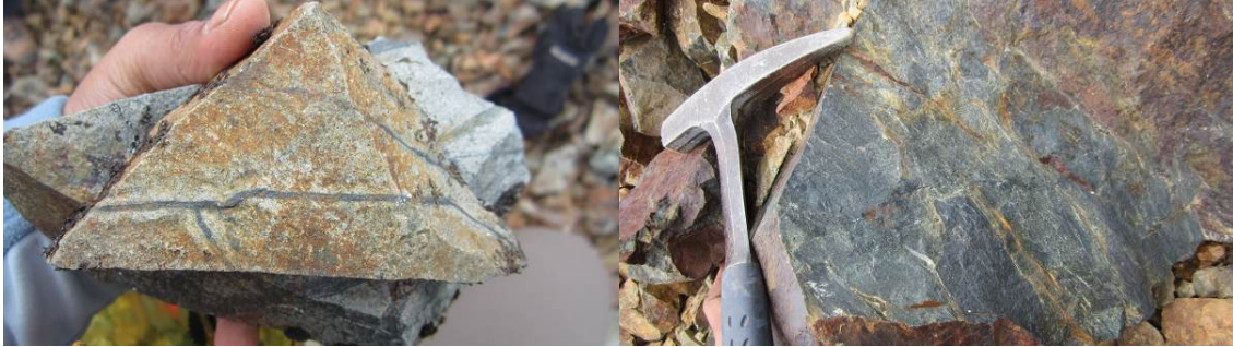
Photo 14, L. Magnetite veins on andesite volcanics (?). Photo 15, R. A blob of magnetite in pervasively chlorite-magnetite-altered andesite volcanics (?)
