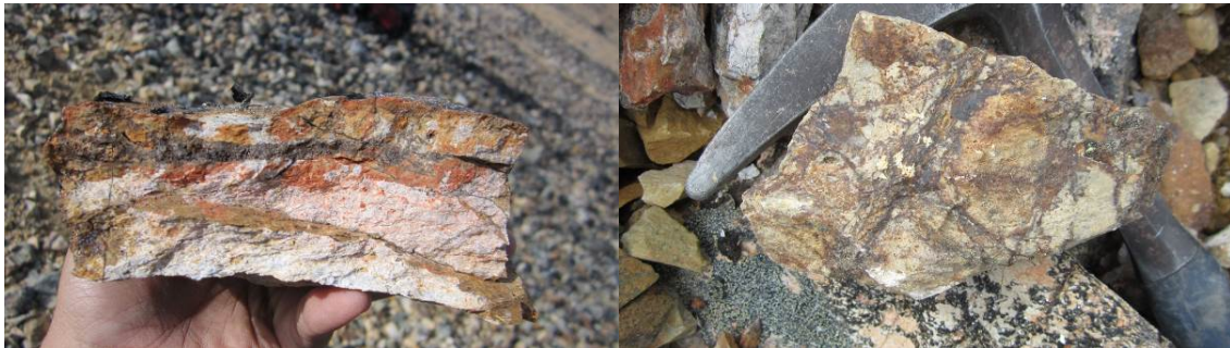
Photos 11-12. Muscovite-altered volcanics(?) with quartz-hematite veins found on the central part of the Silica Ridge (R) and on the eastern side of the ridge (Sample 363).
