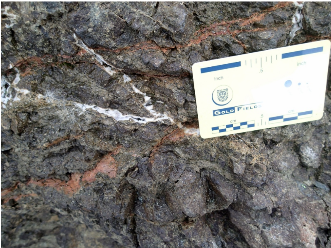
Figure 4: Rock Photo of the Porphyry. Note hematite altered fractures cross-cut by discontinuous, chalcidonic quartz veining.
