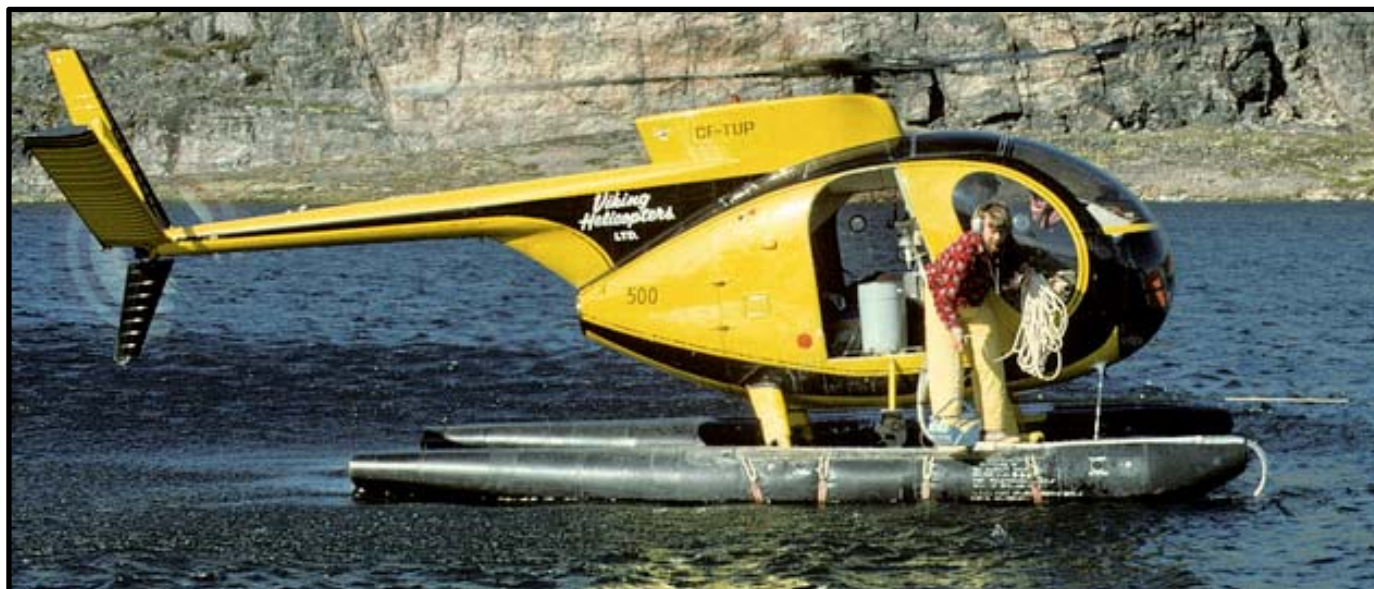
Figure 9. Typical method of lake sediment sampling
