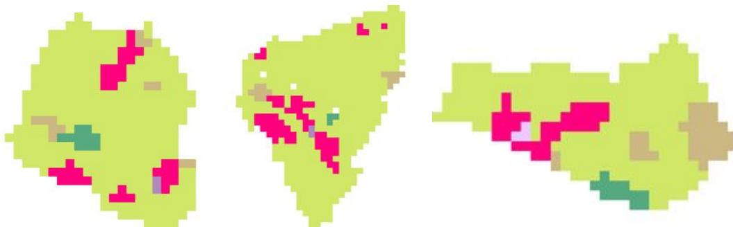
Figure 5: TIMA images illustrating discrete mica inclusions in K-feldspar indicating limited sericitic alteration of the feldspar reducing problematic flotation of the Cu-sulphides.
