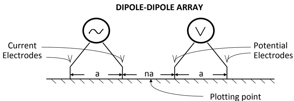
The lines run in a due northeast direction ( $45^{\circ}\text{E}$ ) and are 100 meters apart. The electrode separation, or 'a' spacing, and reading interval was chosen to be 30 meters read to 12 separations, which is the 'na' in the above diagram, for all three lines. The 12 separations give a theoretical depth penetration of about 200 meters, or 650 feet.
