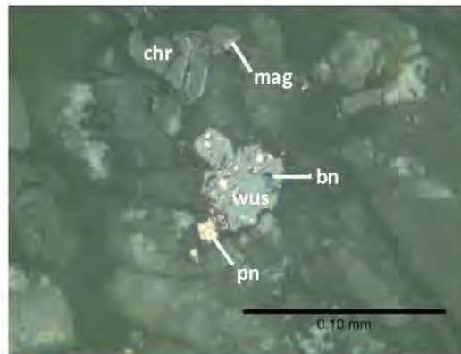
Fig. 2: Photomicrograph of a small pod of pentlandite (pn), wustite (wus), and bornite (bn). Wustite replaces pentlandite. Chromite (chr) with magnetite (mag) rims around grain boundaries appears above. Photo taken in plane polarized reflected light.
