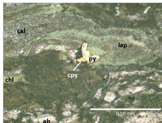
Figure 2: Photomicrograph of chalcopyrite (cpy) and pyrite (py) occurring together within a lapilli (lap). The lapilli are composed of a calcite (cal)-limonite core and chlorite (chl) rim. Photo taken in plane polarized transmitted and reflected light.
