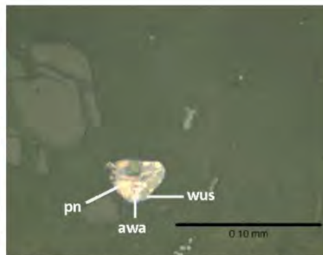
Fig. 2: Photomicrograph of a small pod of mixed and intergrown pentlandite (pn), awaruite (awa), and wustite (wus) with a generally brecciated and cracked texture hosted serpentine. Photo taken in plane polarized reflected light.
