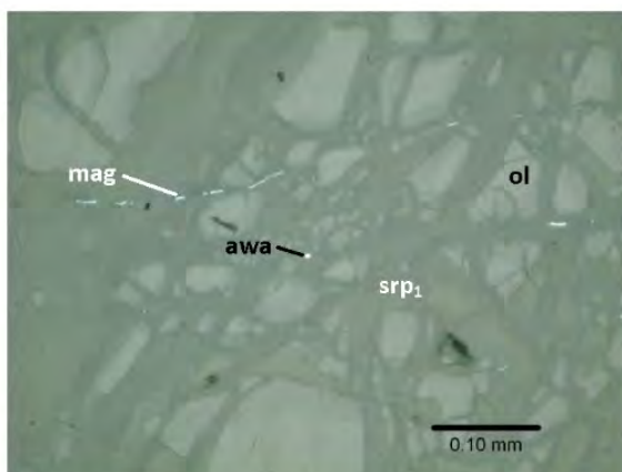
Fig. 1: Photomicrograph of awaruite (awa) and magnetite (mag) in serpentine 1 (srp 1 ) cutting and replacing olivine (ol). Photo taken in plane polarized reflected light.
