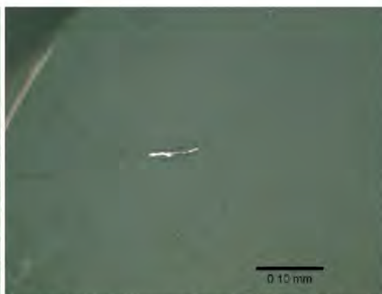
Fig. 2: Photomicrograph of an elongated grain of awaruite (white grain) embedded in serpentine 3 vein cutting serpentine 2. Photo taken in plane polarized reflected light.
