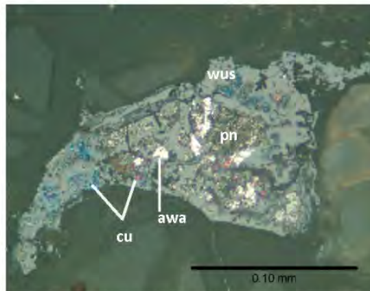
Fig. 2: Photomicrograph of a small pod of pentlandite (pn), native copper (cu), awaruite (awa), and wustite (wus) with a generally brecciated and cracked texture hosted serpentine. Photo taken in plane polarized reflected light.
