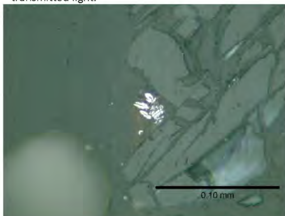
Fig. 1: Photomicrograph of serpentine 3 (srp 3 ) veins cutting a serpentine 2 (srp 2 ) vein on the left, and a serpentine 3 vein being offset by a serpentine 2 vein. It is difficult to tell which set of serpentine veins overprints which, or if they are simply intergrown cogenetically. A serpentinized orthopyroxene grain (opx srp ) occurs at the bottom of the photo in the serpentine 2 vein. Photo taken in plane polarized transmitted light.
