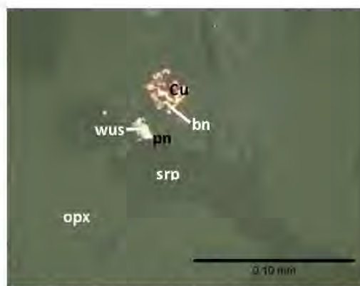
Fig. 2: Photomicrograph of a small pod of mixed and intergrown pentlandite (pn) and wustite (wus) hosted in fractured and serpentinized orthopyroxene (opx). Native copper (Cu) and bornite (bn) are found within an altered orthopyroxene grain. Photo taken in plane polarized reflected light.
