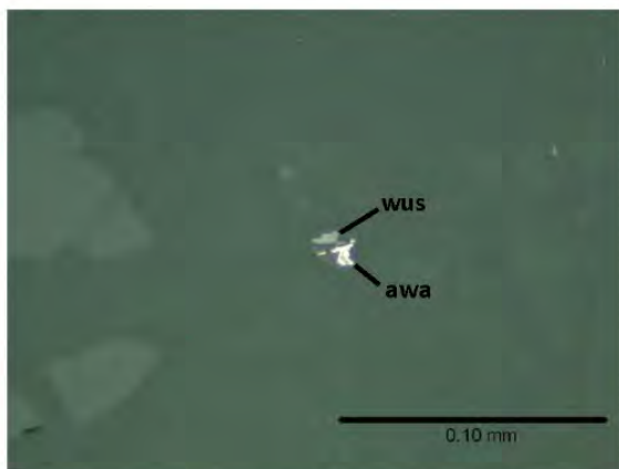
Fig. 1: Photomicrograph of a grain of awaruite (awa) associated with wustite (wus) in serpentine 2. Photo taken in plane polarized reflected light.
