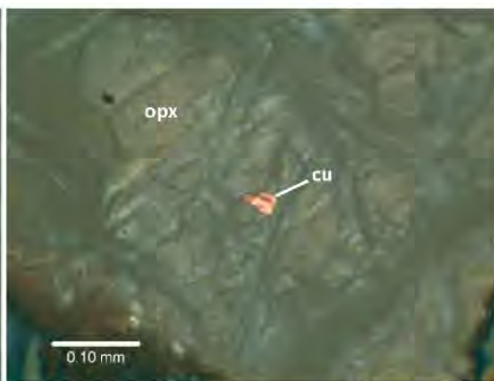
Fig. 2: Photomicrograph of an irregular grain of native copper (cu) found in serpentine 1 alteration of orthopyroxene (opx). Photo taken in plane polarized reflected and transmitted light.
