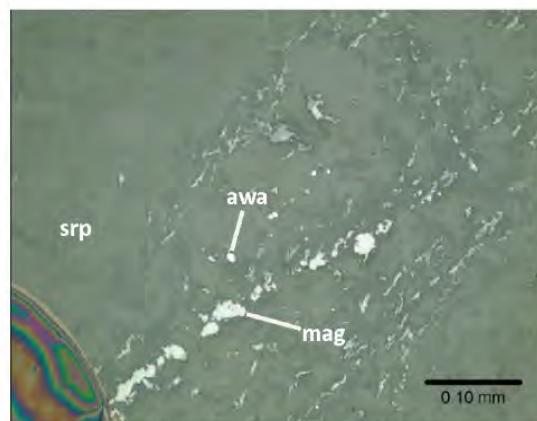
Fig. 2: Photomicrograph of trace awaruite (awa) disseminated in serpentine (srp) and associated with strings of granular magnetite (mag). Photo taken in plane polarized reflected light.
