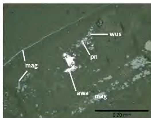
Fig. 2: Photomicrograph of anhedral awaruite (awa) associated with stringy magnetite (mag) and wustite (wus)-replacing-pentlandite (pn) in a zoned serpentine vein. Photo taken in plane polarized reflected light.
