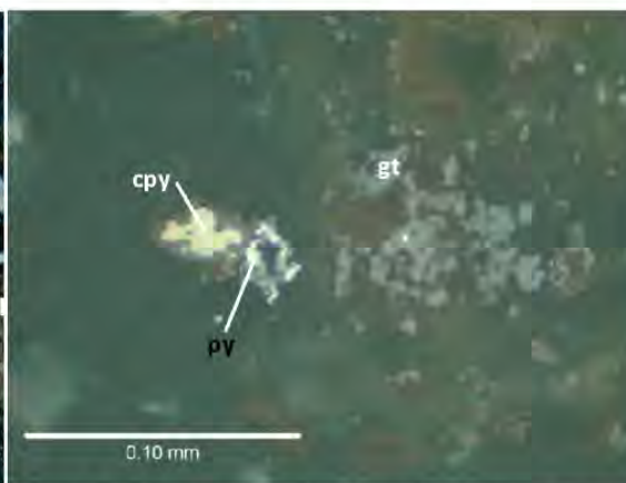
Figure 2: Photomicrograph of irregular chalcopyrite (cpy) and pyrite (py) rimmed by goethite (gt) replacement. Photo taken in plane polarized reflected light.
