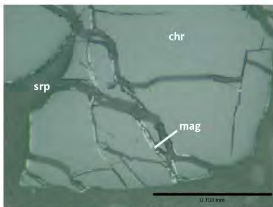
Fig. 1: Photomicrograph of subhedral chromite (chr) with fractures which host veiny magnetite (mag) alteration associated serpentine (srp). Photo taken in plane polarized reflected light.
