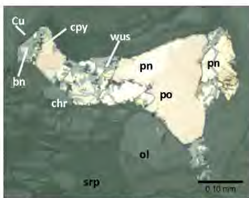
Fig. 1: Photomicrograph of a brecciated pod associated with serpentine alteration in olivine (ol). Pentlandite (pn), chalcopyrite (cpy), bornite (bn), and native copper replace pyrrhotite (po) and pentlandite (pn), and wustite (wus) fills the cracks. A single grain of chromite (chr) is associated with the sulphides. Photo taken in plane polarized reflected light.
