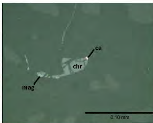
Fig. 2: Photomicrograph of native copper (cu) embedded in actinolite (act) replacing monticellite (mtc). Photo taken in plane polarized reflected light.
