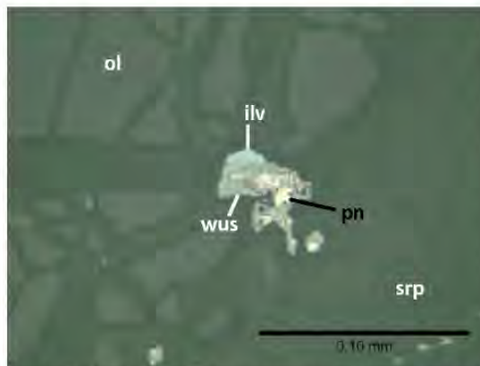
Fig. 2: Photomicrograph of pentlandite (pn), wustite (wus), and ilvaite (ilv) with a generally brecciated texture associated with serpentine 1 (srp) in fractured olivine (ol). Pentlandite is rimmed and replaced by wustite, and wustite fills the fractures between pentlandite, which is then overprinted by ilvaite. Photo taken in plane polarized reflected light.
