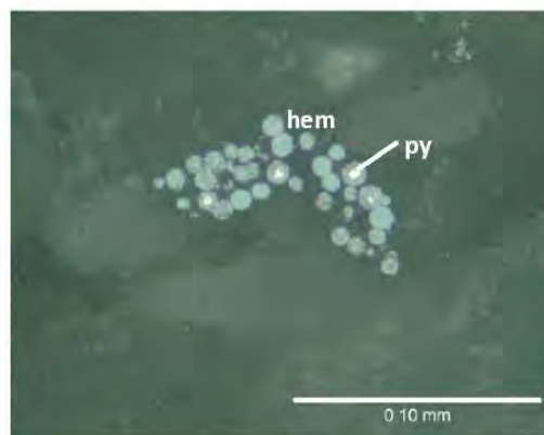
Figure 2: Photomicrograph of pyrite (py) balls rimmed and replaced by hematite (hem). Photo taken in plane polarized reflected light.
