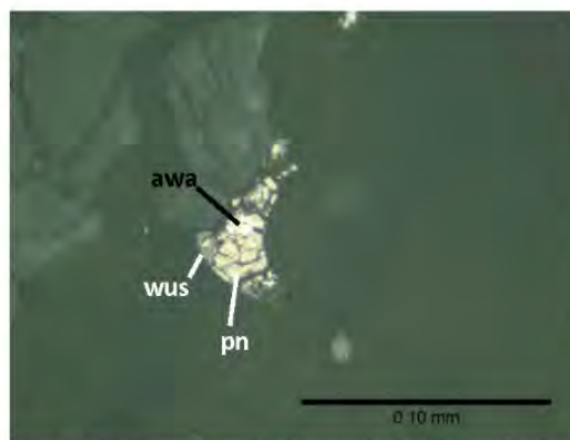
Fig. 2: Photomicrograph of a pod of pentlandite (pn), wustite (wus), and awaruite (awa) and sphene, associated with fractured olivine in serpentine 1. Awaruite occurs as an anhedral mass between pentlandite. Photo taken in plane polarized reflected light.
