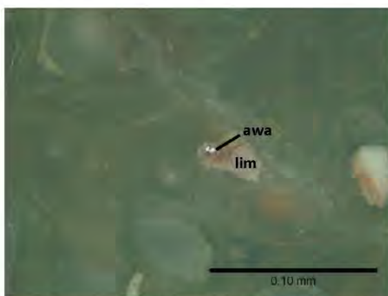
Fig. 1: Photomicrograph of a grain of awaruite (awa) associated with limonite (lim) in serpentine 1. Photo taken in plane polarized reflected light.
