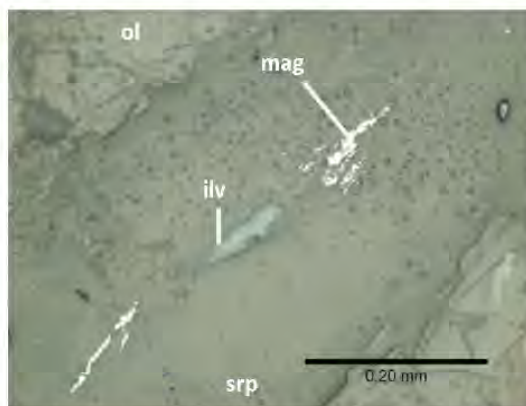
Fig. 2: Photomicrograph of ilvaite (ilv) associated with stringy magnetite (mag) in a serpentine 1 vein (srp). Photo taken in plane polarized reflected light.
