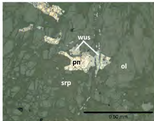
Fig. 2: Photomicrograph of a small 0.2 mm long pod of pentlandite (pn) with a generally brecciated and cracked texture being replaced by wustite (wus) hosted in fractured and serpentinized olivine (ol). The wustite is intimately associated with the serpentine vein cutting the pentlandite. Photo taken in plane polarized reflected light.
