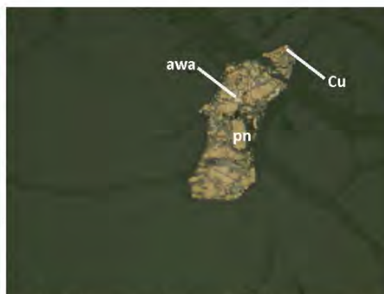
Fig. 2: Photomicrograph of a small 0.1 mm long pod of mixed and intergrown pentlandite (pn), awaruite (awa), and native copper (Cu) with a generally brecciated and cracked texture hosted in fractured and serpentinized olivine. Photo taken in plane polarized reflected light.
