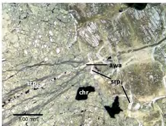
Fig. 1: Photomicrograph of several generations of serpentine alteration. Serpentine 1 is characterised as the pervasive, green flooding serpentine which partially to completely replaces host rock olivine and orthopyroxene. Serpentine 2 (srp 2 ) is characterised by grey veins with minor magnetite. Serpentine 3 (srp 3 ) is characterized by colourless serpentine veins hosting bladed magnetite. Serpentine 4 is not visible in this photo. Serpentine 5 (srp 5 ) is characterised by pale brown to beige serpentine, minor ovoid calcite, and minor cubic magnetite. Photo taken in plane polarized transmitted light.
