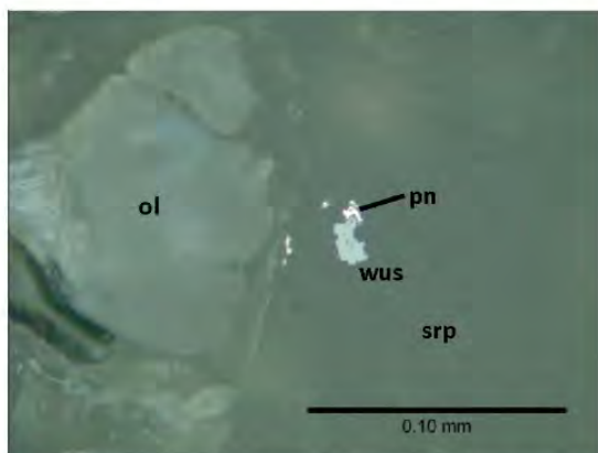
Fig. 1: Photomicrograph of a small pod of pentlandite (pn) and wustite (wus) in serpentine (srp) alteration along the edge of olivine (ol). Photo taken in plane polarized reflected light.
