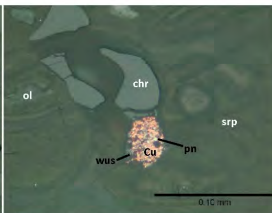
Fig. 2: Photomicrograph of an isolated grain of native copper (Cu) associated with chromite (chr) within serpentine (srp) which cuts olivine (ol). Photo taken in plane polarized reflected light.
