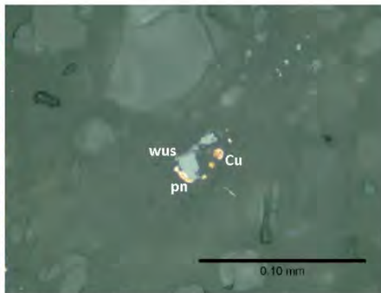
Fig. 2: Photomicrograph of a small pod of wustite (wus) with pentlandite (pn) and native copper (Cu) in serpentine 1. Photo taken in plane polarized reflected light.
