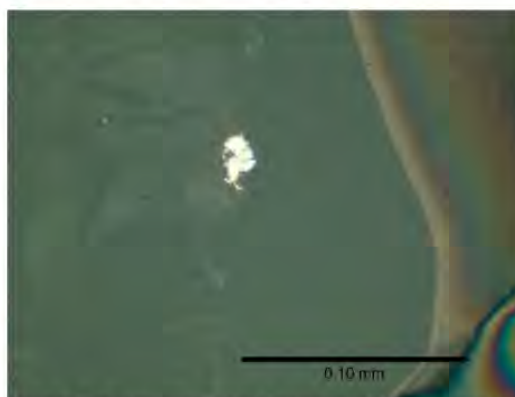
Fig. 2: Photomicrograph of a grain of awaruite embedded in serpentine. Photo taken in plane polarized reflected light.
