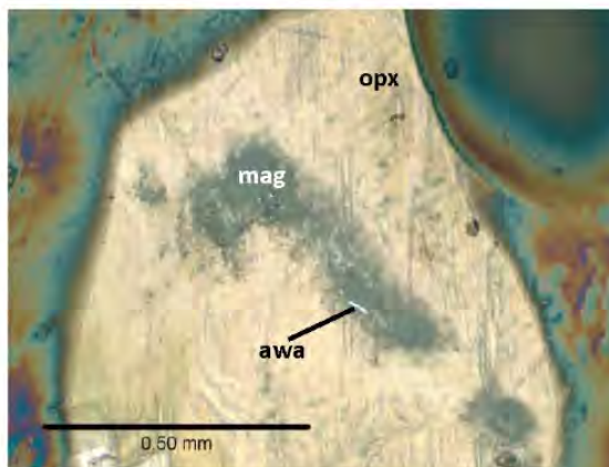
Fig. 2: Photomicrograph of an elongated grain of awaruite (awa) with magnetite (mag) in serpentinized orthopyroxene (opx). Photo taken in plane polarized transmitted and reflected light.
