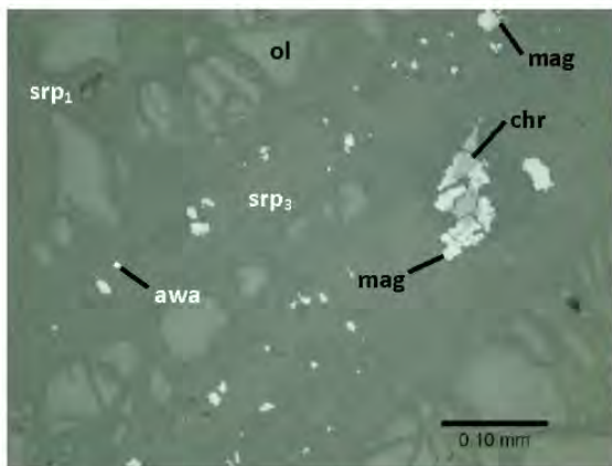
Fig. 1: Photomicrograph of serpentine 3 (srp 3 ) veins cutting serpentine 1 (srp 1 ). These veins contain cubic to subhedral magnetite (mag) grains along vein selvages, and a primary chromite (chr) grain that is altered to magnetite around grain boundaries. Photo taken in plane polarized reflected light.
