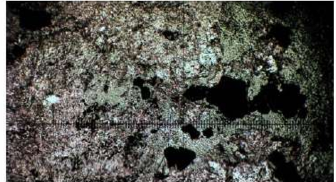
B. Photomicrograph showing quartz chlorite and sericite. XPL. Each whole measure on the scale bar is 0.4mm.
