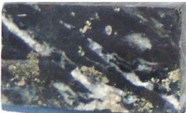
A. Prepared section off-cut. The white minerals are calcite and quartz, the dark minerals are chlorite. Field of view is approximately 26mm x 46 mm.
