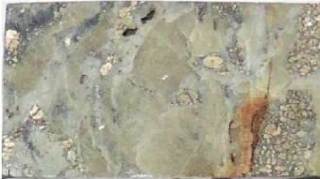
A. Prepared section off-cut. Grey mineral is muscovite and quartz, transparent grains are quartz veins. Field of view is approximately 26mm x 46 mm.
