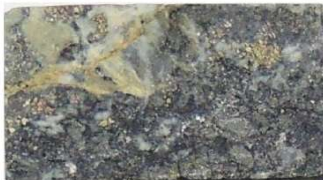
A. Prepared section off-cut. White-translucent minerals are quartz, and muscovite, and dark mineral is pyroxene. Field of view is approximately 26mm x 46 mm
