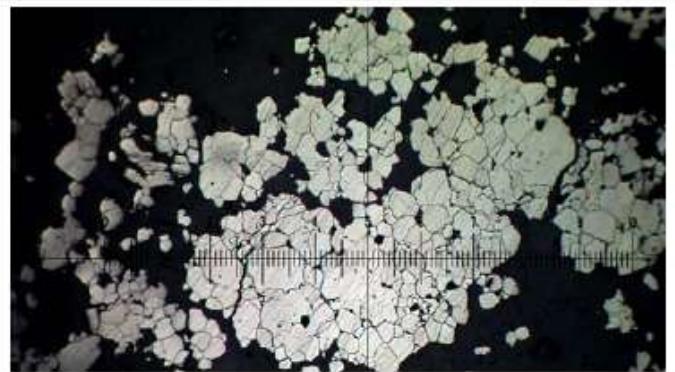
D. Photomicrograph showing pyrite aggregate. RL. Each whole measure on the scale bar is 0.4mm.
