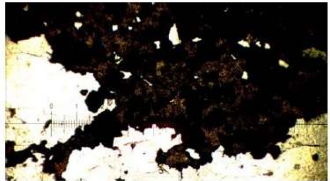
B. Photomicrograph showing sphalerite and quartz. XPL. Each whole measure on the scale bar is 0.4mm.
