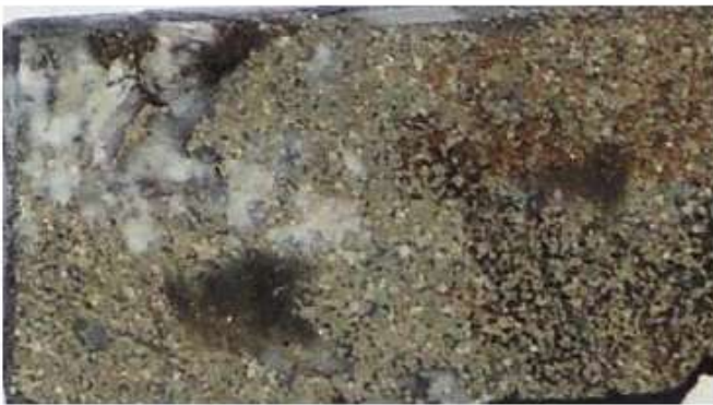
A. Prepared section off-cut. The white minerals are albite and quartz, the metallic mineral is pyrite. Field of view is approximately 26mm x 46 mm.
