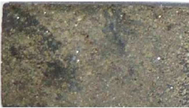
A. Prepared section off-cut. The white minerals are plagioclase and quartz, the dark mineral is hornblende. Field of view is approximately 26mm x 46 mm.
