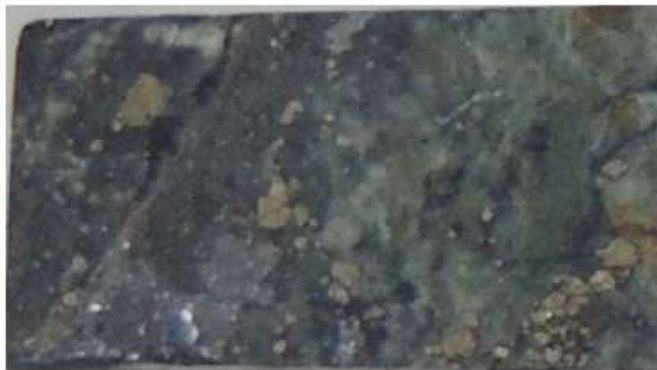
A. Prepared section off-cut. The white mineral quartz, the dark minerals are muscovite and chlorite. Field of view is approximately 26mm x 46 mm
