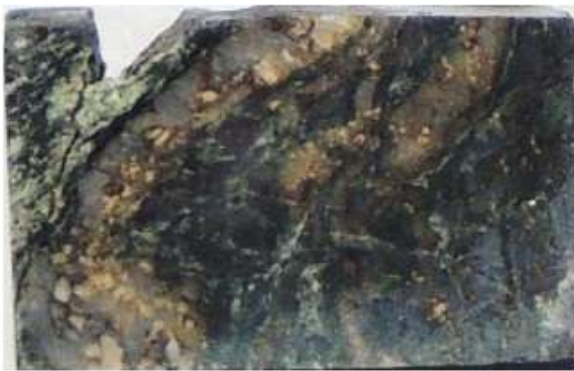
A. Prepared section off-cut. The white minerals are feldspar and quartz, the dark minerals are pyroxene and hornblende. Field of view is approximately 26mm x 46 mm.
