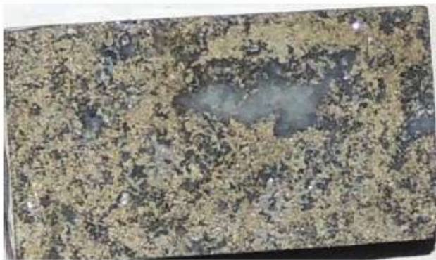
A. Prepared section off-cut. The white minerals are quartz, the metallic mineral pyrite. Field of view is approximately 26mm x 46 mm.
