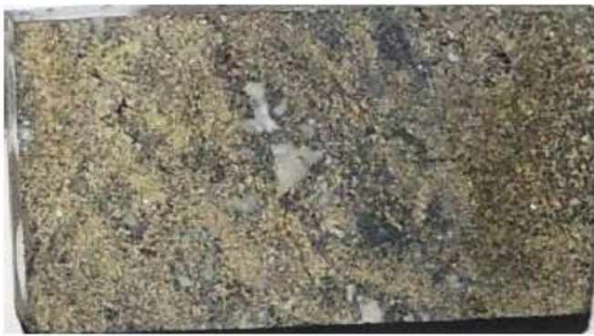
A. Prepared section off-cut. The white minerals are feldspar and quartz, the dark minerals are pyroxene and hornblende. Field of view is approximately 26mm x 46 mm.
