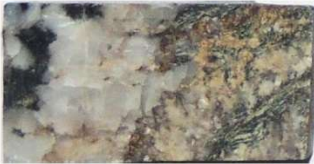
A. Prepared section off-cut. The white minerals (left) are quartz, the white-yellow minerals (right) are carbonate, muscovite and chlorite. Field of view is approximately 26mm x 46 mm.
