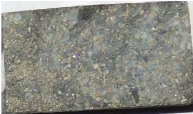
A. Prepared section off-cut. The white minerals are plagioclase and quartz, the dark mineral is hornblende. Field of view is approximately 26mm x 46 mm.
