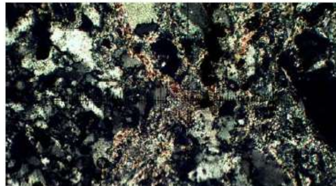
B. Photomicrograph showing quartz, sericite and pyrite. XPL. Each whole measure on the scale bar is 0.4mm.
