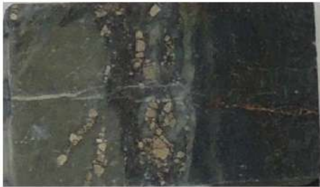
A. Prepared section off-cut. Contact between mudstone (left) and volcanic flow (right) with pyrite. Field of view is approximately 26mm x 46 mm
