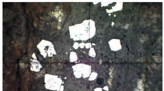
D. Photomicrograph showing pyrite. Partial cross-polarized RL. Each whole measure on the scale bar is 0.4mm.
