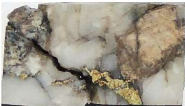
A. Prepared section off-cut. The white minerals are quartz, the fragment on the right is carbonate and the fragment on the left is albite, chlorite and quartz. Field of view is approximately 26mm x 46 mm.
