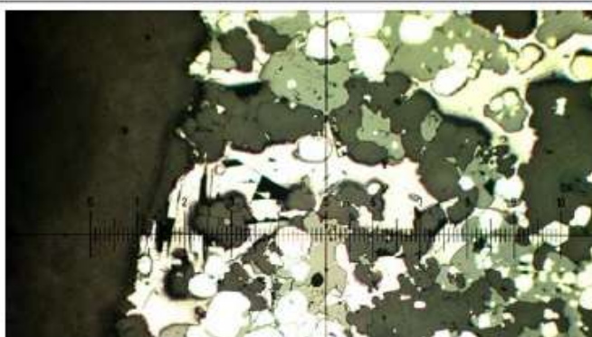
D. Photomicrograph showing pyrite, chalcopyrite and galena. RL. Each whole measure on the scale bar is 0.4mm.
