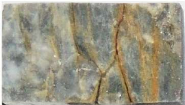
A. Prepared section off-cut. The dark grey areas are sericite and quartz. The white areas are zones of quartz aggregates. Field of view is approximately 26mm x 46 mm
