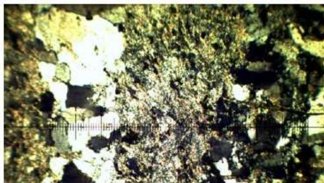
B. Photomicrograph showing quartz and sericite. XPL. Each whole measure on the scale bar is 0.4mm.
