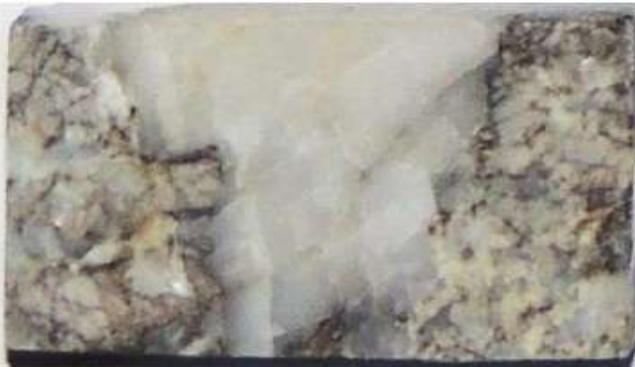
A. Prepared section off-cut. The white minerals are quartz, the off-white mineral are carbonate minerals. Field of view is approximately 26mm x 46 mm.
