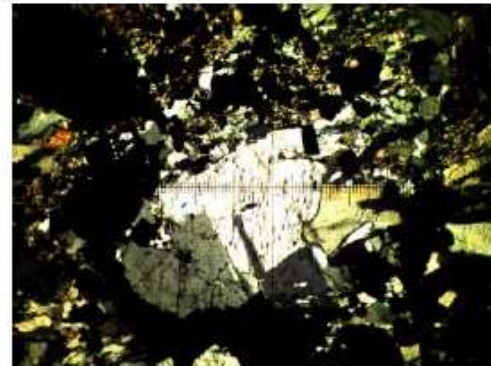
B. Photomicrograph showing quartz, albite, and sericite. XPL. Each whole measure on the scale bar is 0.4mm.
