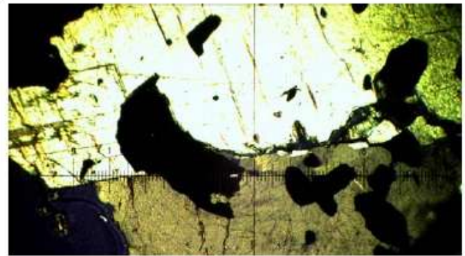
B. Photomicrograph showing carbonate and quartz. XPL. Each whole measure on the scale bar is 0.4mm.
