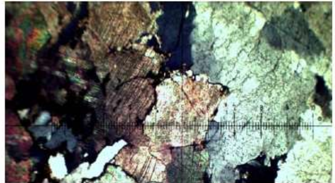
B. Photomicrograph showing quartz and carbonate minerals. XPL. Each whole measure on the scale bar is 0.4mm.
