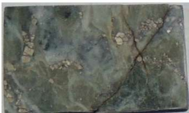
A. Prepared section off-cut. The whitish area is the silica flooded and the brownish area is the metamorphosed mudstone. Field of view is approximately 26mm x 46 mm.
