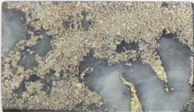
A. Prepared section off-cut. The white minerals are quartz and the metallic mineral is pyrite. Field of view is approximately 26mm x 46 mm.
