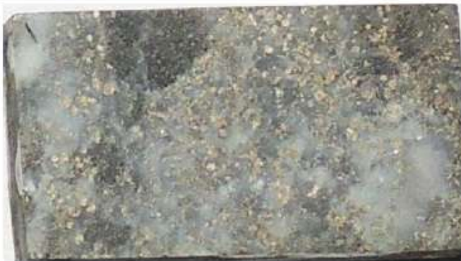
A. Prepared section off-cut. The white minerals are quartz, the dark minerals are sericite and quartz, the metallic areas are pyrite. Field of view is approximately 26mm x 46 mm.
