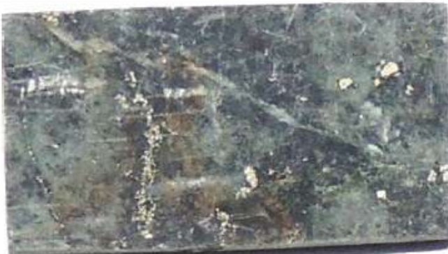
A. Prepared section off-cut. The darker areas are chlorite rich the lighter areas are sericite rich. Field of view is approximately 26mm x 46 mm.
