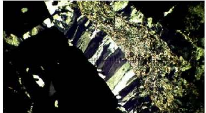
B. Photomicrograph showing colloform quartz, fine-grained muscovite and quartz matrix. XPL. Each whole measure on the scale bar is 0.4mm.
