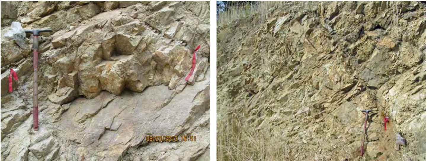
Fig. 16 Two photos detailing 3 of 4 measured samples collected along structures in the BH sill. Left photo has 0648 left of hammer, 0647 to right is a cm-sized white quartz vein with trace limonite. Rt photo is a brittle fault viewed about along strike; channel sample 0645 sampled reddish limonitic fault gouge. The fault orients 018 46 SE.
