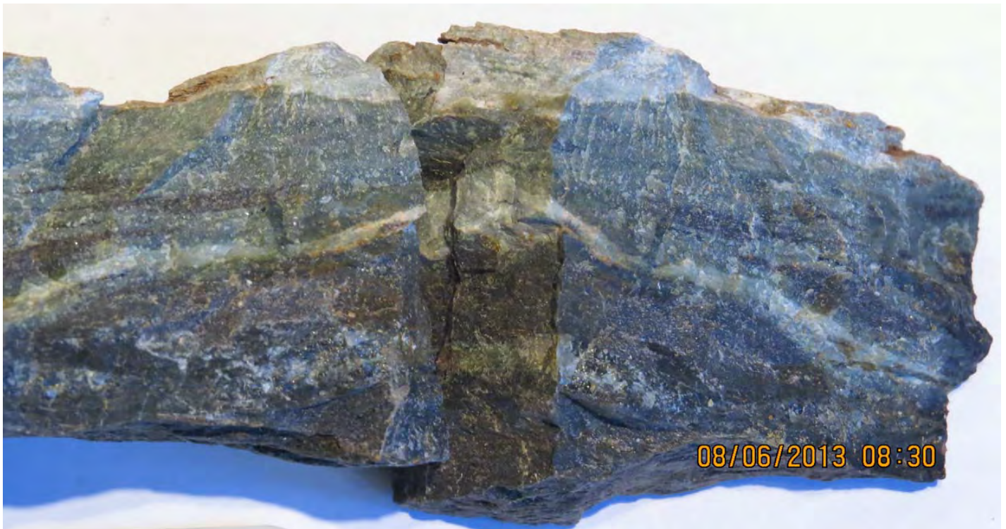
Fig. 12 Close-up photo of 0228D hand specimen, dark green and maroon-purple banded calc-silicate skarn with sparse sulphides.
