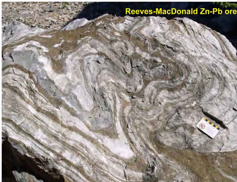
Fig. 10 Banded and doubly-folded lead-zinc-silver ore from the Reeves MacDonald deposit, photo card has cm divisions. Photo from Paradis & Simandl (2007).
