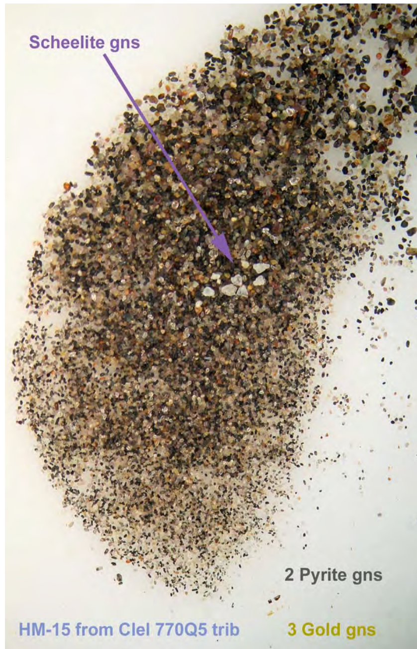
Fig. 26 Overview of the many gns of HM-15 Clel 770Q5 trib HM concentrate, a goethite-forsterite/diopside mineral assemblage. A close-up of the scheelite gns is below. In the medium size sand fractions HM-15 is 1st rank in spessartine with 5,000 {5,883} gns, 5th rank in scheelite 30 {35} gns and 4th rank in Chromite or Hercynite or Cr-spinels 40 {47} gns. It is anom in Calculated Gold in the 'total' bulk silt 17.79 ppb (Map H-04) though it is not anomalous in VG gns with 5 recovered = 0 Reshaped + 3 Modified + 2 Pristine, a total of {6} if standardized to 10 kg. Clel 770Q5 trib basin is a target for a spessartine + scheelite + native Au bearing skarn system.
