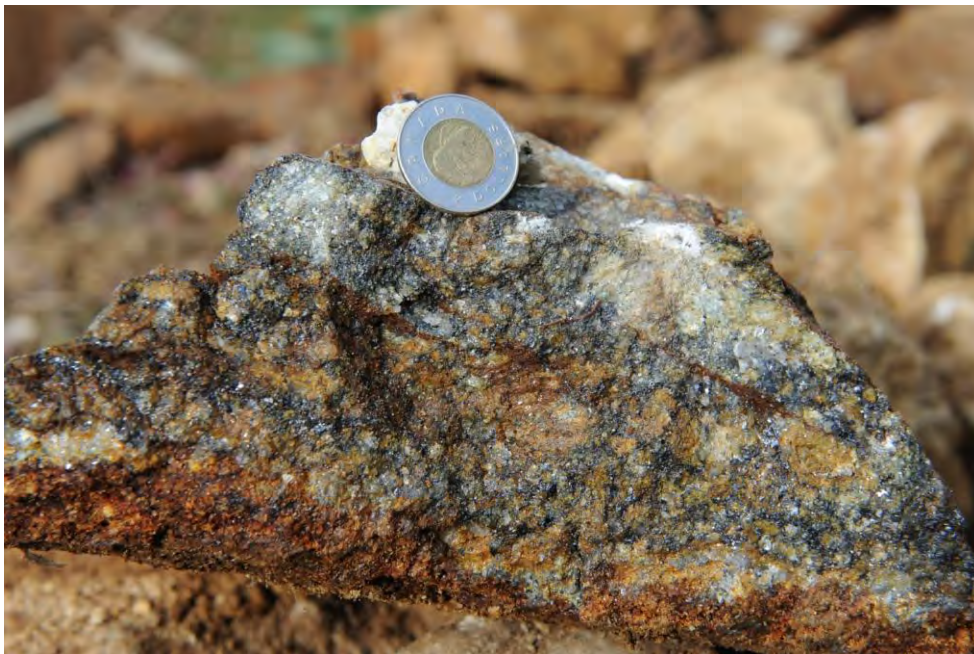
Figure 7.2: Coarse sphalerite in glassy-quartz and diopside-bearing calcsilicate characterizes the style of mineralization.
