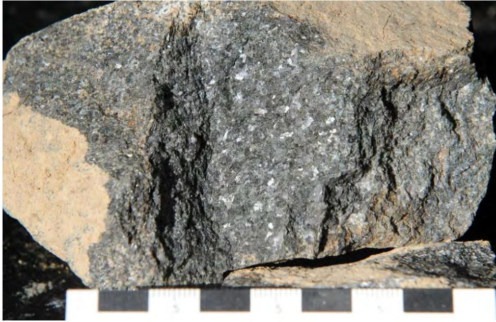
Figure 7.1: Massive, coarse-crystalline black sphalerite sample from subcrop excavated in test pit1 (1.5 m deep) dug on a 492 ppm Zn anomaly in Ah (humus) soil. Excavated bedrock consists of diopside-bearing calcsilicate and marble, which is host to Zn-rich mineralization 1.4 km farther south (in the trench zone) along the regional strike.
