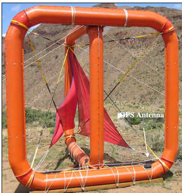
Figure 5: ZTEM base station receiver coils.
