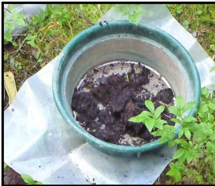
Figure 12. A 4mm mesh sieve used in the field to separate organic material from Ah soils and larger rocks from B-C soils.
