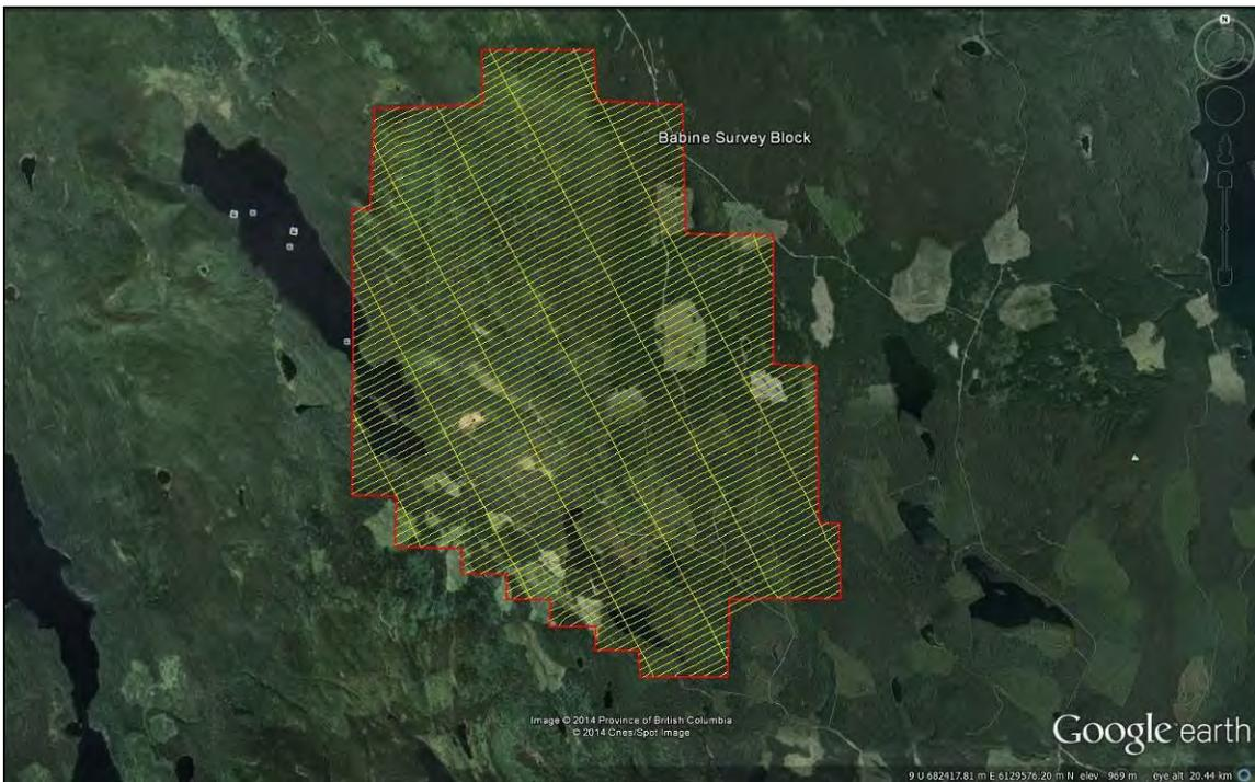
Figure 4: Plane View – Babine survey block with actual survey and tie lines outlined in yellow, and the survey block boundary in red.
