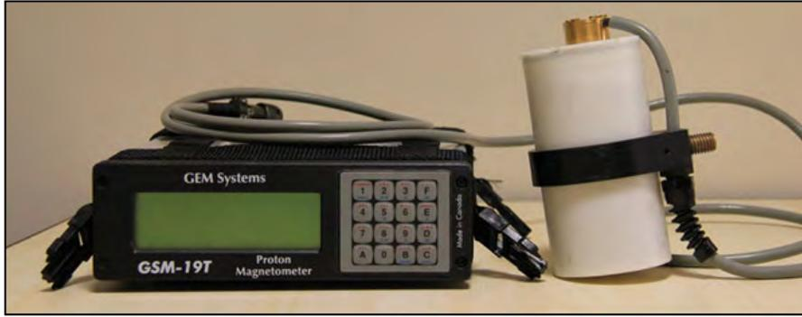
Figure 14: GEM GSM-19T proton precession magnetometer.
