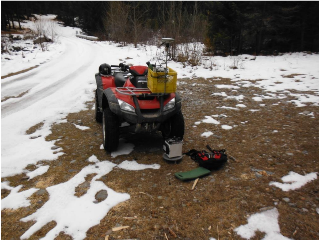
Figure 3. Typical Gravity Station Setup.
