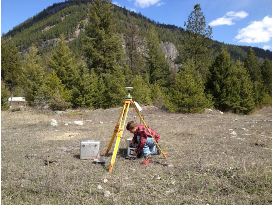
Figure 8. Operator taking a gravity reading at a field GPS base station.
