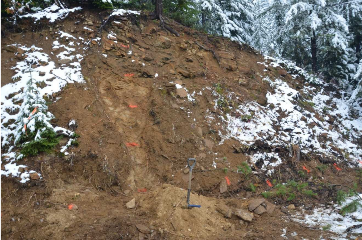
Figure 6 'Weather Station' zone – 5 metre (top to bottom) continuous exposure across gently dipping graphite-bearing stratigraphy
