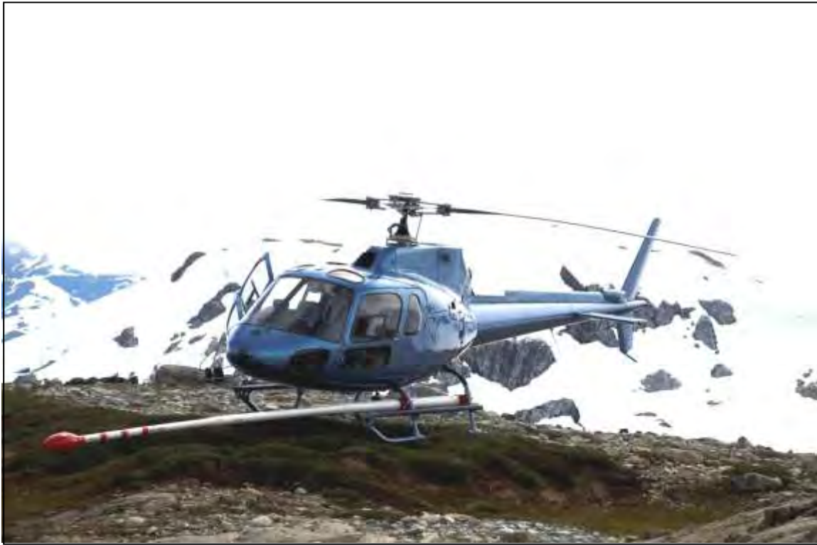
Figure 10: Eurocopter AS350 equipped with mag stinger for magnetic data acquisition.
