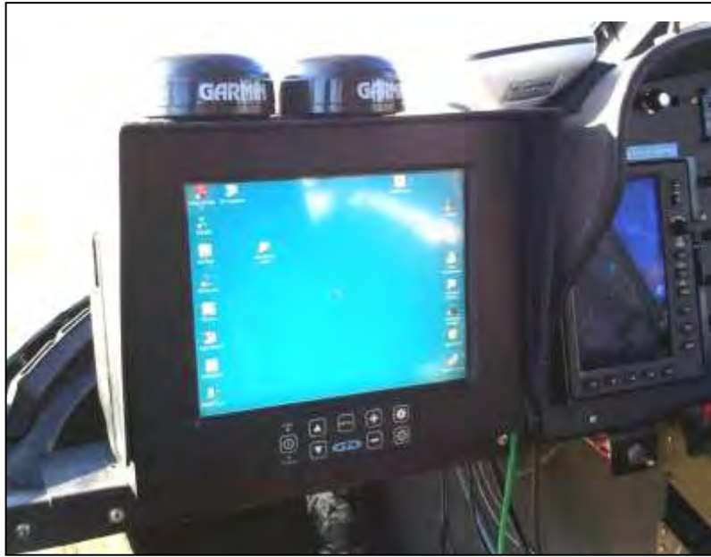
Figure 11: AGIS operator display installed in the Eurocopter AS350B2.
