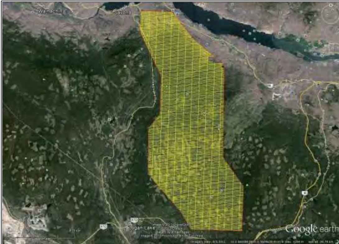
Figure 4: Plane View – Rabbit North survey block with actual survey and tie lines outlined in yellow, and the survey block boundary in red.
