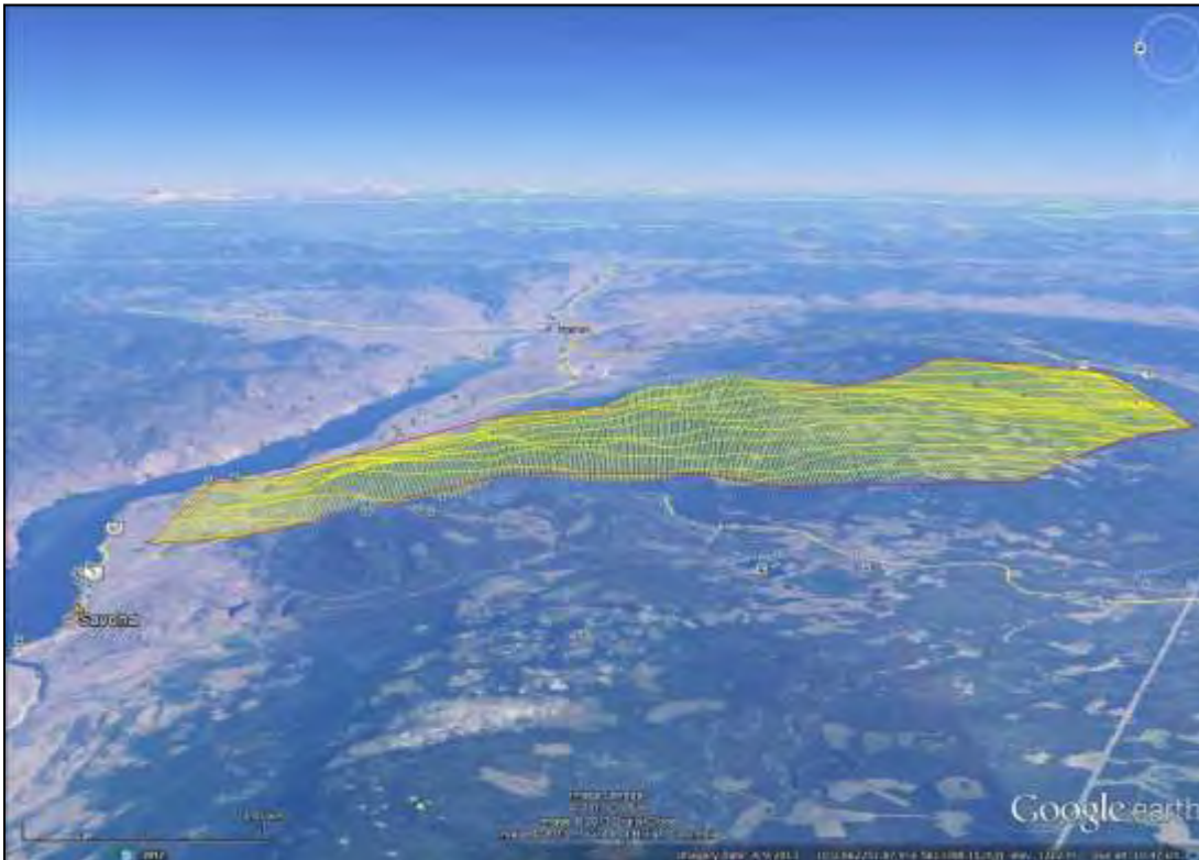
Figure 5: Terrain View – Rabbit North survey block with actual survey and tie lines outlined in yellow, and the survey block boundary in red.
