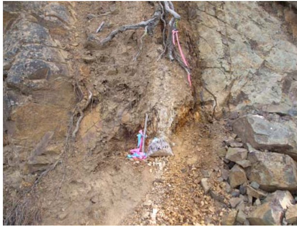
Photo 6: Shear zone, with chip sample 937RTR024 across 50 cm, and which ran 3,637 ppb Au and 452 Cu.
