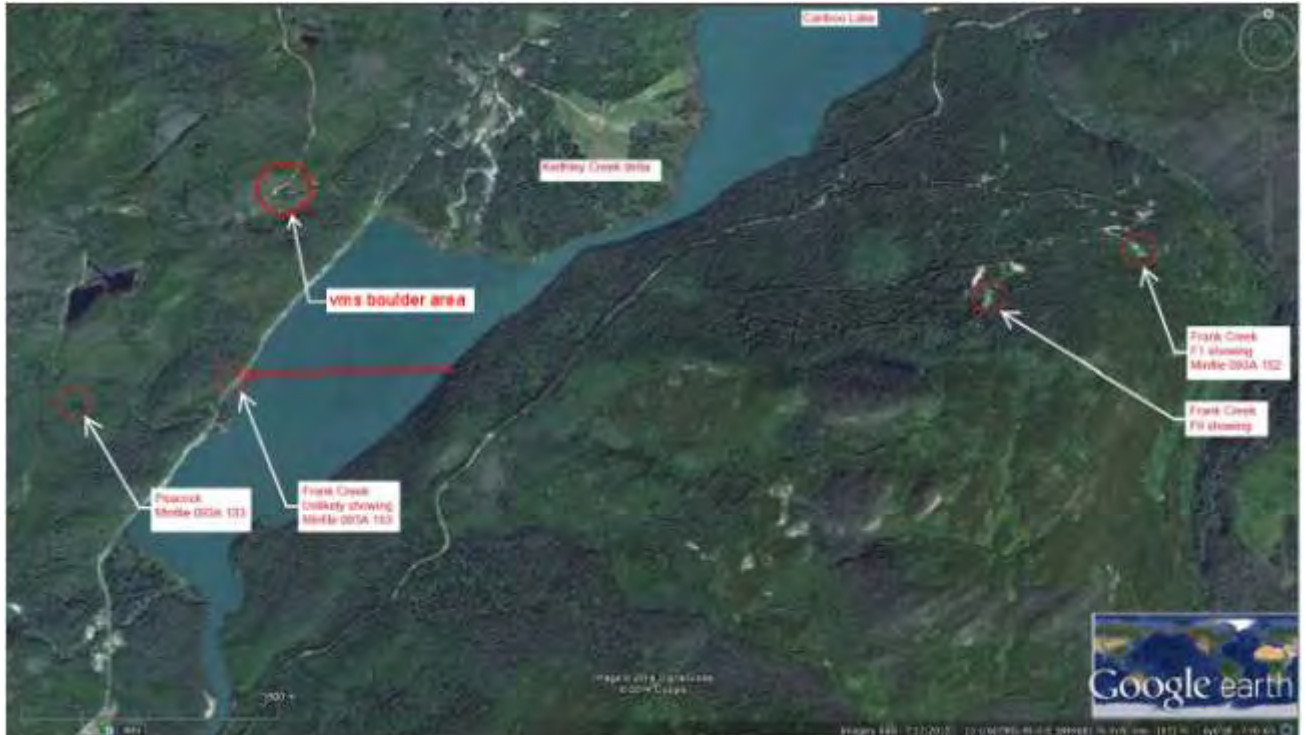
Figure No. 11. Satellite photo of approximately the same area at Frank Creek as in Figure No. 10. An east-west topographic lineament, located on the south side of the Frank Creek F1 and F9 showings, extends westward toward the Unlikely showing. The lineament is plainly evident over the land area across the centre of the photo and is partly indicated by a red line drawn only over the lake. A portion of the Unlikely showing outcrop has intense shearing (see Figure No. 12) indicating an east-west fault with a vertical dip which may be related to the above lineament. The proposed E-W fault may pre-date the NE-SW fault (or joint) occupying the Cariboo Lake valley as the latter fault line shows no significant displacement in an E-W direction. Likewise, the proposed E-W fault also appears not to be displaced as its line crosses the Cariboo Lake valley undisturbed. This, and the regional geology, suggest no great strike-slip movement occurred along the NE-SW line. It is possible the Peacock, Unlikely and vms boulder mineral occurrences to the west are equivalent to the F1 and F9 occurrences at Frank Creek, displaced by an E-W fault.
