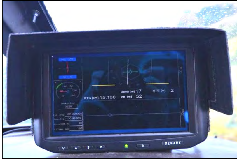
Figure 15: Pilot Guidance Unit.
