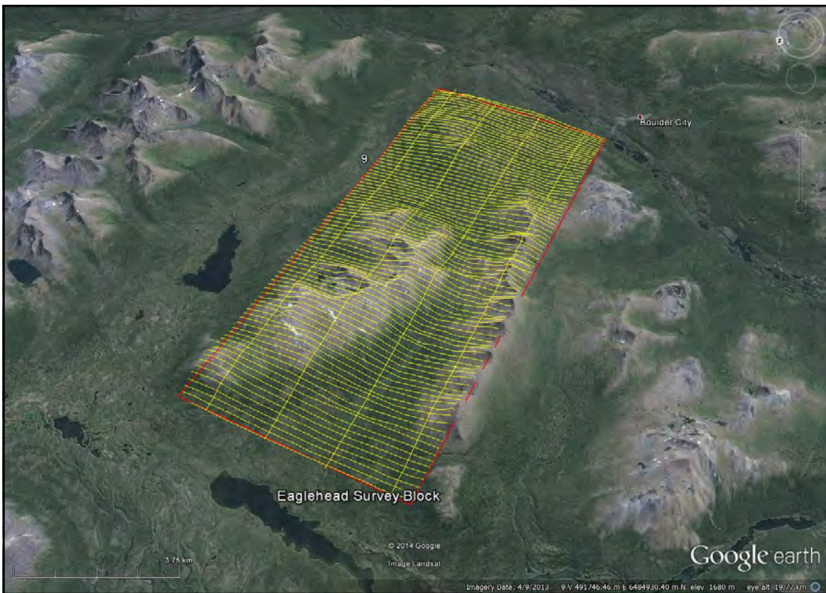
Figure 4: Terrain View – Eaglehead survey block with actual survey and tie lines outlined in yellow, and the block boundary in red.
