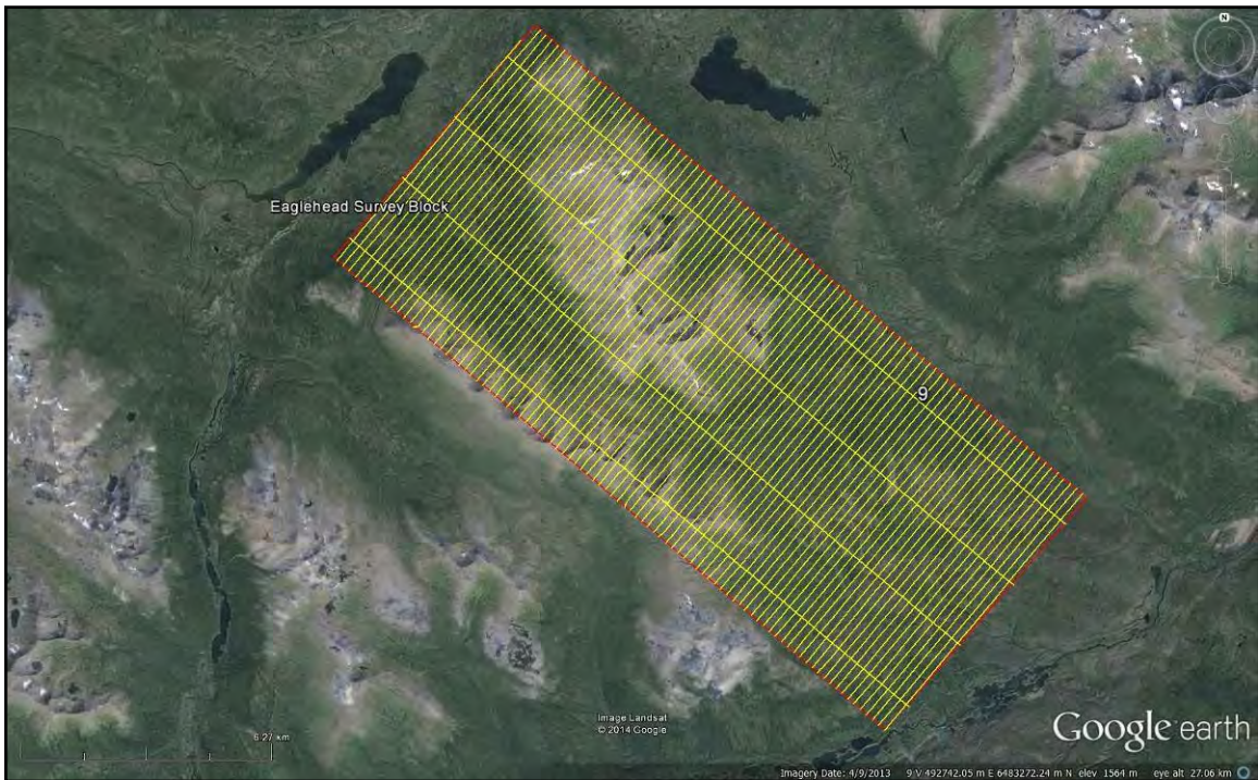
Figure 3: Plan View – Eaglehead survey block with actual survey and tie lines outlined in yellow, and the block boundary in red.
