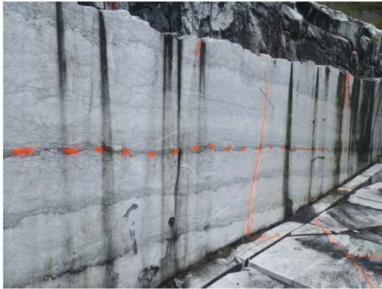
Figure 8: Grey stylolitic banding in sawn quarry face.
