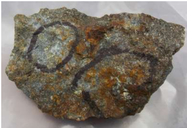
Figure No. 1A Rollie Creek property. Area B1, Location RCL-10b. Semi massive sulphide with chalcopyrite.
