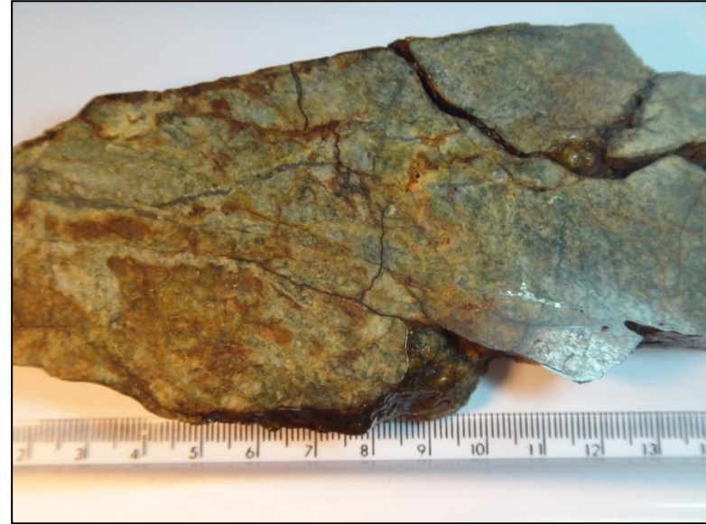
Plate 1 b: Handspecimen 1593158, showing nature of brecciation (sample is 16 cm long)
