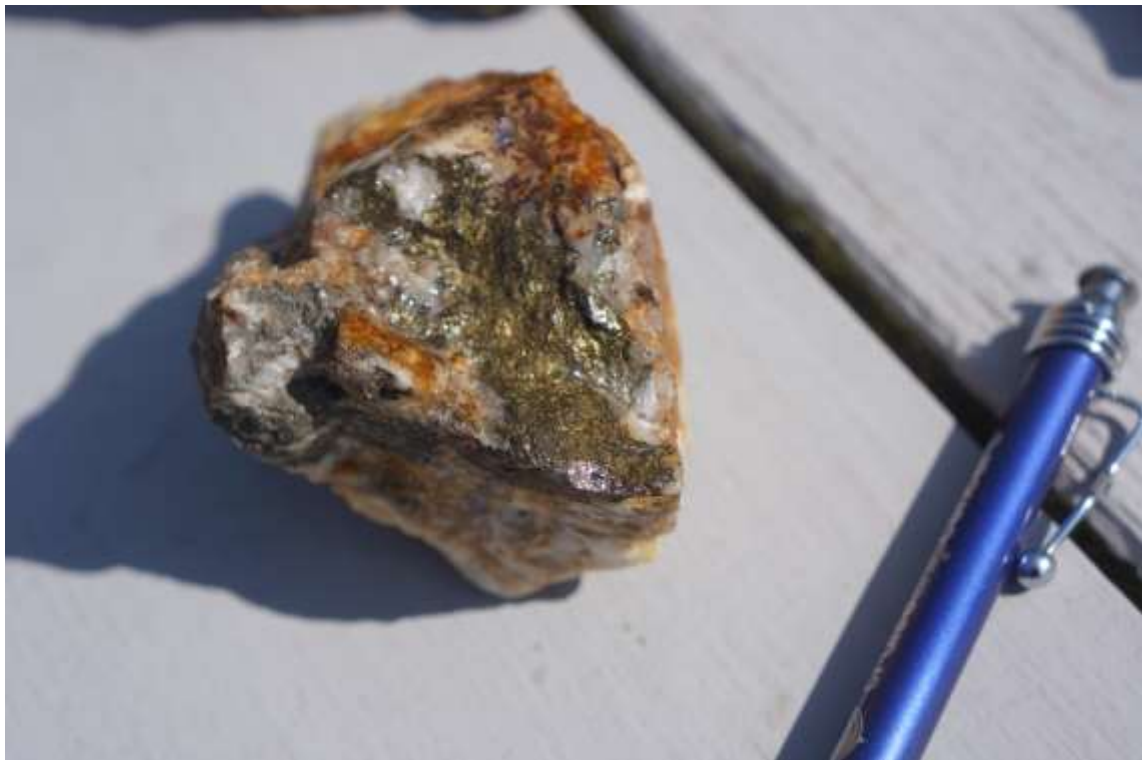
FIGURE 7: SAMPLE FROM "ADIT ZONE" VISIBLE GOLD AND PYRRHOTITE. SAMPLE IS FROM MR YAKIMISHYN'S PERSONAL COLLECTION.
