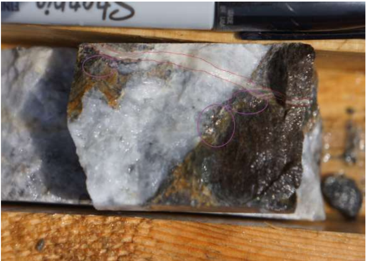
FIGURE 8: THICKER QUARTZ CARBONATE VEIN CUT BY FINER GRAINED BARREN QUARTZ CARBONATE VEIN (OUTLINED IN RED). PURPLE CIRCLES HIGHLIGHT PYHROTITE, CHALCOPYRITE, GOLD MINERALIZATION ALONG THE EDGE OF THICKER VEIN. (HOLE OP-04-05 Box 7 42.5M)
