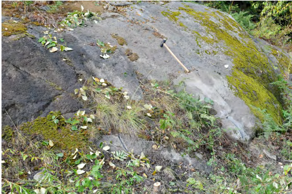
Figure 7.6: Roadside exposure of LBDR showing overall competence, internal homogeneity, resistance to weathering, and overall structural integrity. The 1.5 m long sledge handle provides scale and saw cuts are present at bottom right of the exposure. Based on these observations we surmise that LBDR would pass any tri-axial compression strength tests required for approval as building stone.
