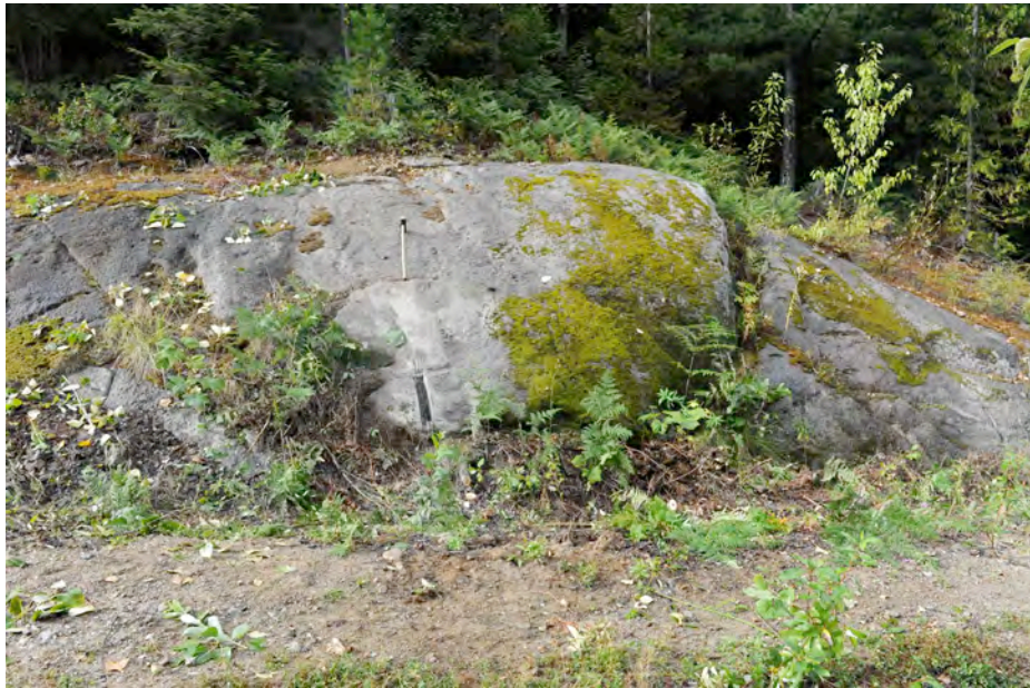
Figure 7.2a: Outcrop exposure of LBDR showing competent, glacially-induced rounding without obvious flaws caused by surface weathering. Sledge for scale, saw cuts at base.
