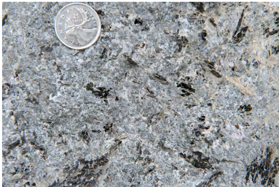
Figure 7.1b: Fresh, broken surface of LBDR showing the distinctive porphyritic texture reflective coloring of feldspar in the matrix. Surfaces are created by breaking along crystal boundaries, not fractures.
