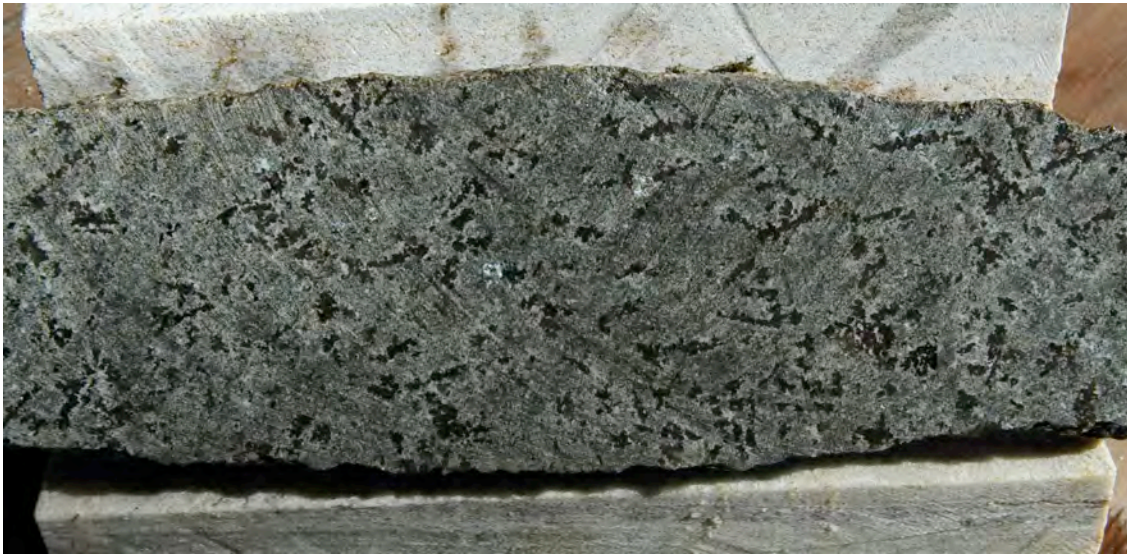
Figure 7.1a: Slabbed sample of LBDR showing porphyritic texture defined by elongate clusters of biotite crystals (black) and highlighted by iridescent reflections from labradorite within the dark grey feldspar matrix.
