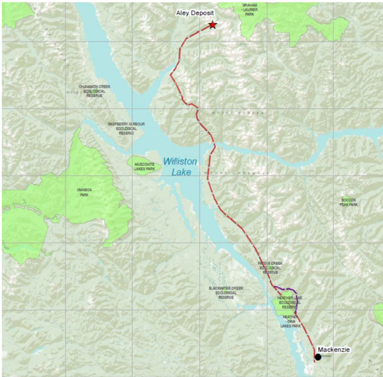
Figure 18.4: Proposed Transmission Line Corridor
