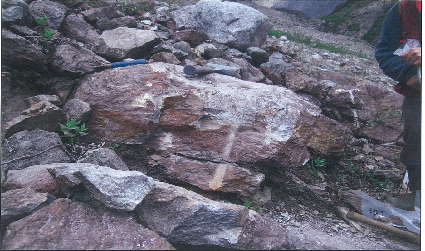
Photo #4: Massive sulphide lens, highly silicified as a block adjacent, in contact with Zone C Hydrothermal Breccia; 50cm chip samples range up to 9.26 g/t Au; 87.2 g/t Ag; 4.14 % Cu; 3.3% Pb; 9.83% Zn
