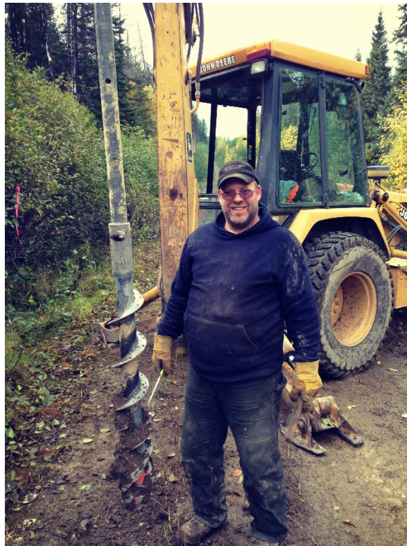
Photo 3 – Operator/pro prospector Jon Rempel cleaning auger flights after collecting deep, above bedrock till sample from ditch on left of photo (pink ribbon).
