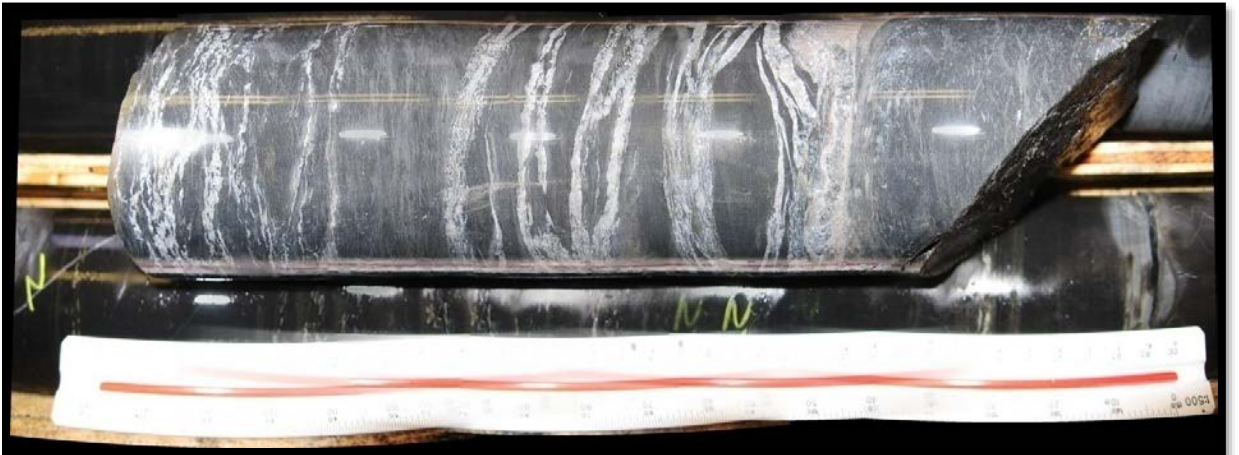
Plate 7-7: Silicification and carbonate veining containing sphalerite in the underlying Silurian siltstone in A-08-63 @ 484m.
