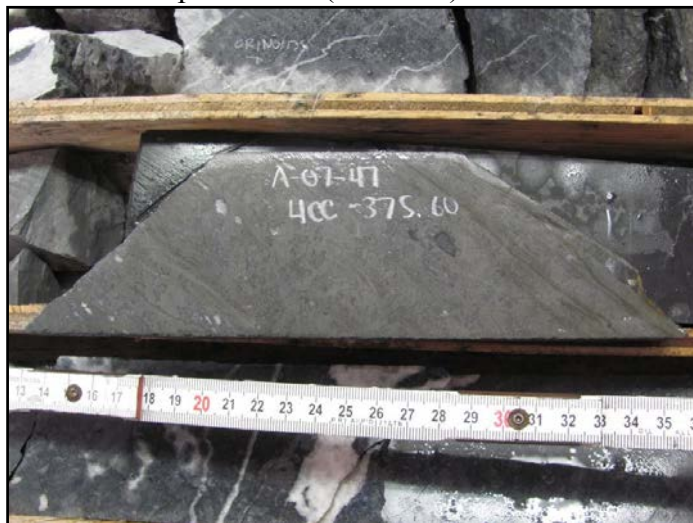
Plate 7-4: High grade sphalerite mineralisation displaying “Mottled” texture in Cardiac Creek Zone facies in A-07-47 @ 375.60.
