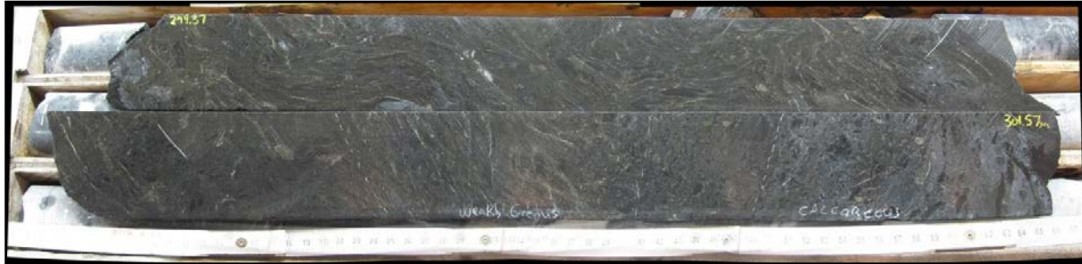
Plate 8-5: Nick style mineralisation in A-10-72 from 299.37 to 301.57m (Photo taken by N. Johnson 2010)
