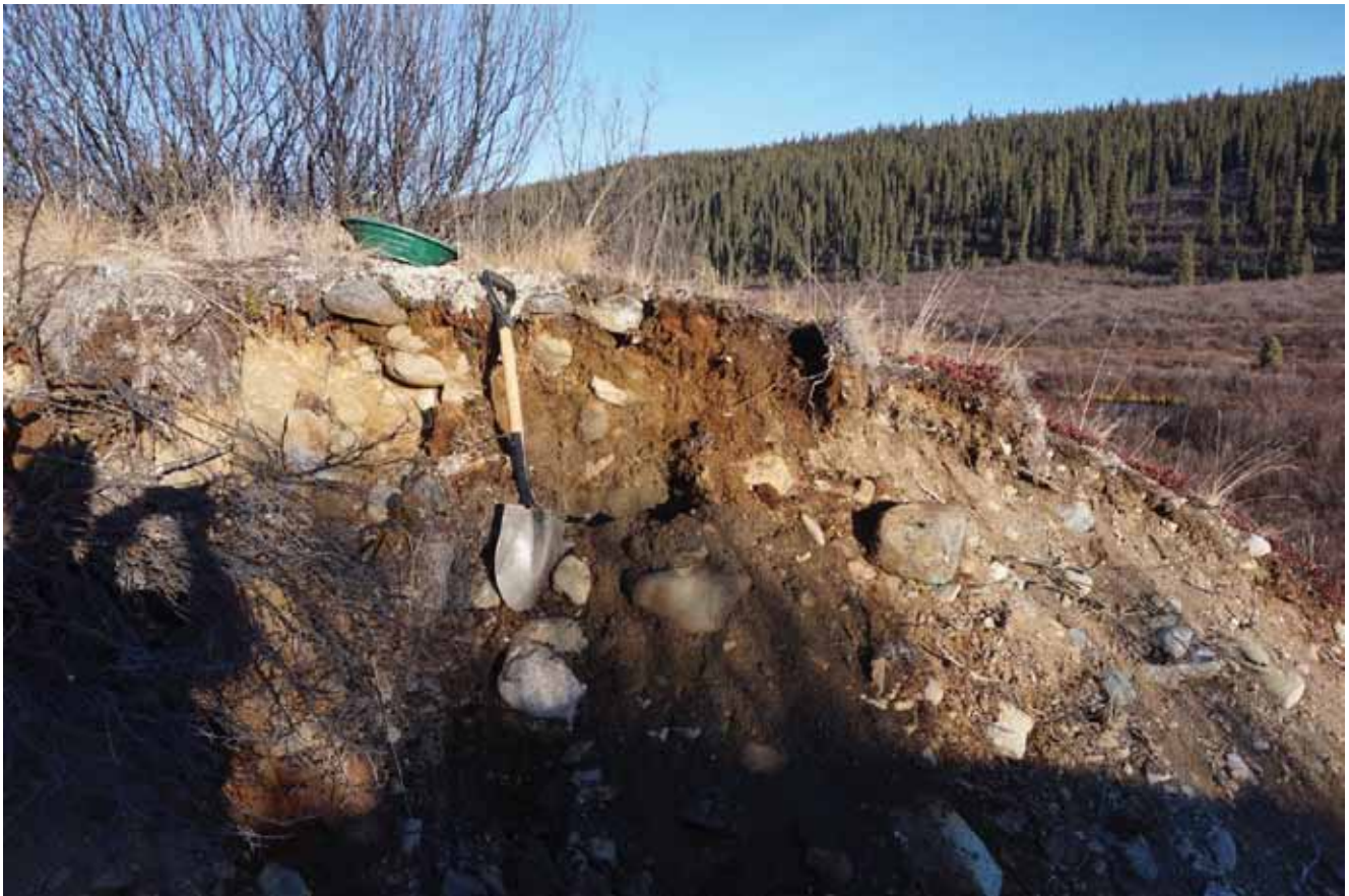
Figure 12. A view to the northeast of the road cut on the FGt3 landform that was used for testing the landform. Note the coarse clast-size in the deposit, which is indicative of a relatively vigorous stream flow at the time of deposition. This gravel contains placer gold.
