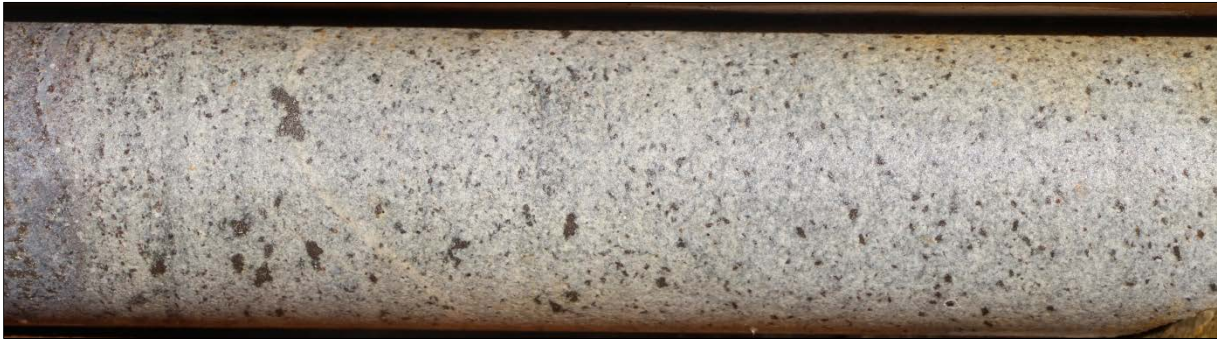
Figure 9: Drill hole C-91-1 at 60m - white to buff coloured arenite, disseminated to blebby pyrrhotite
