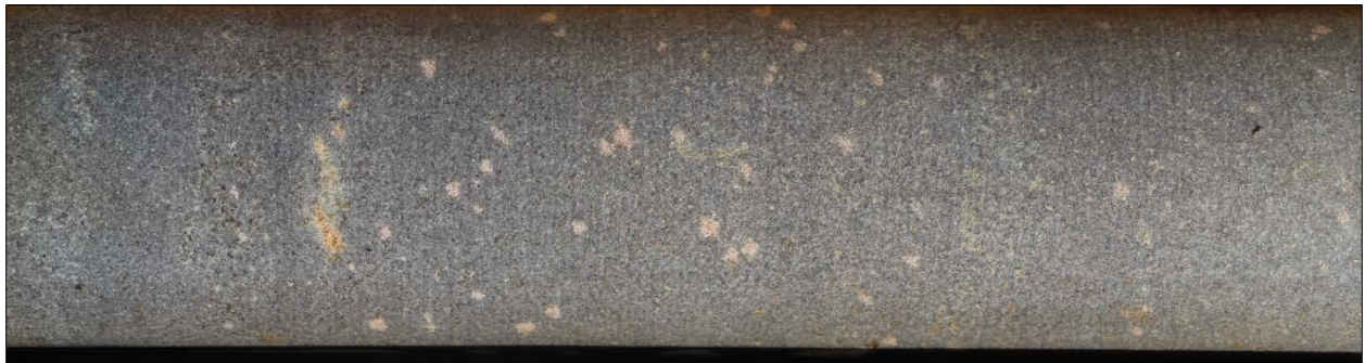
Figure 10: Drill hole C-91-3 at 46m, patchy to blebby garnet alteration within wacke
