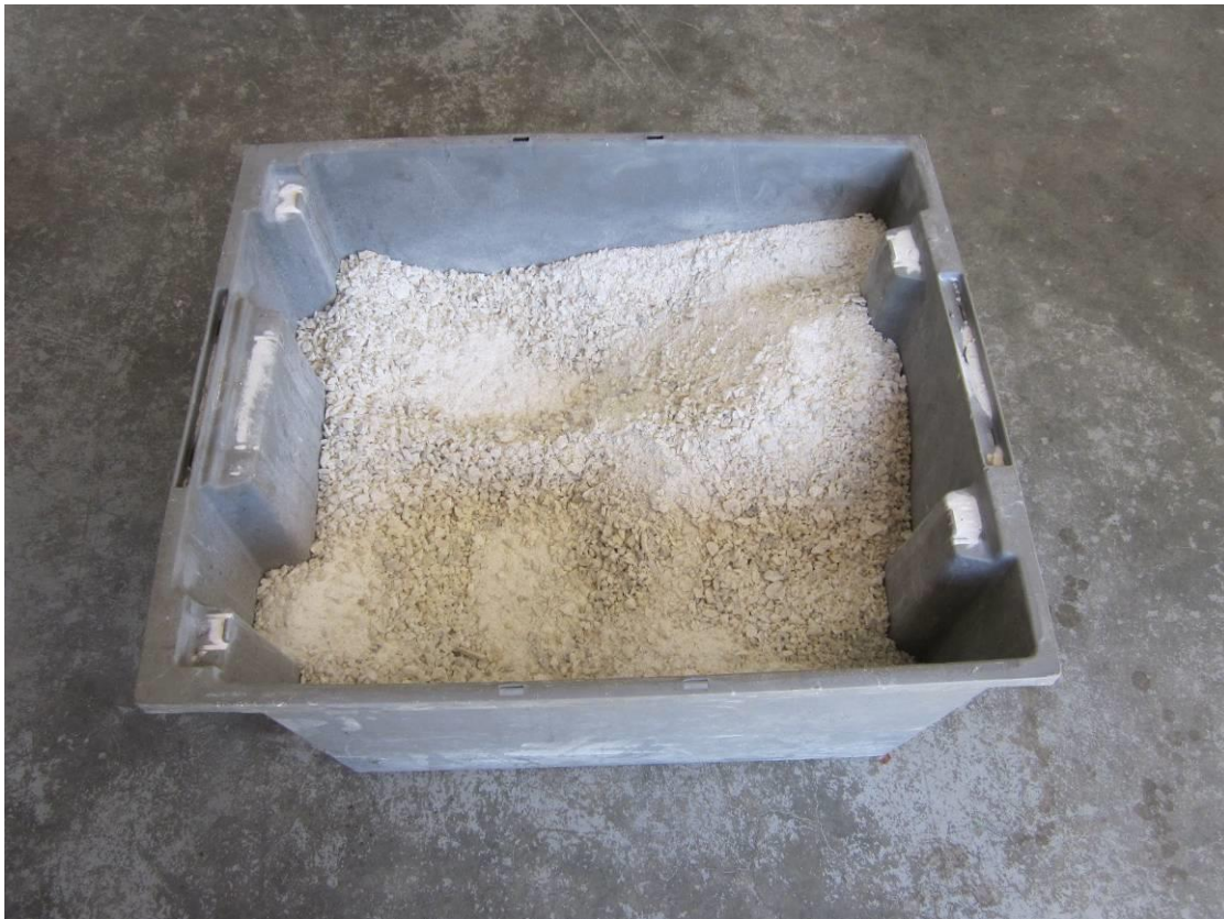
Figure 3. – Photograph of Limestone Sample Used in Calcining Test Work.
