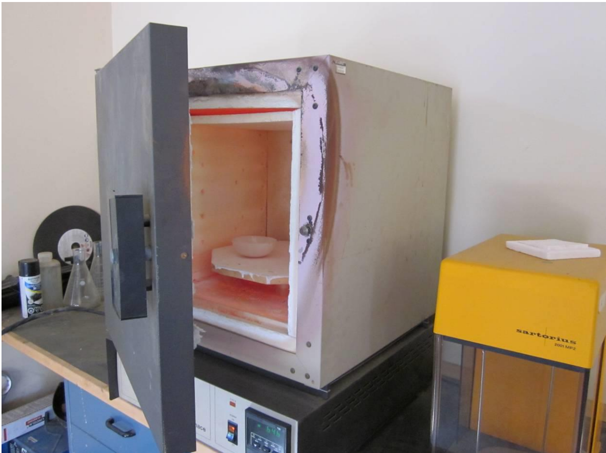
Figure 4. – Thermolyne High Temperature furnace used in Calcining Test Work
